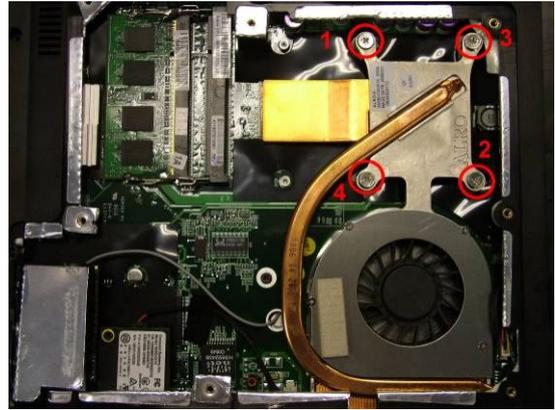
5. Lift out the heatsink assembly.
