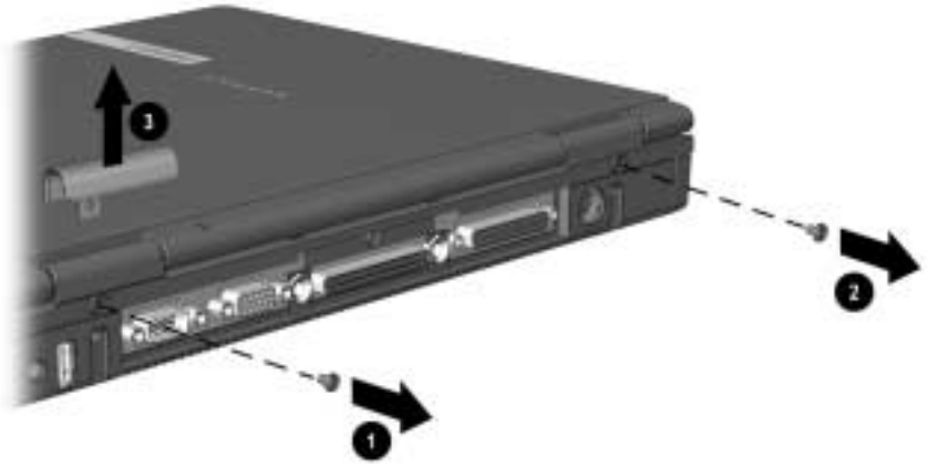
Figure 5-12. Removing the Switch and Hinge Cover Screws
