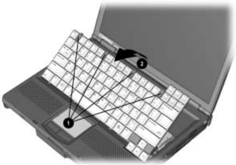
Figure 5-8. Releasing the Keyboard
