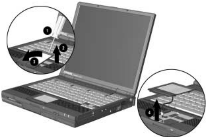
Figure 5-5. Removing the Touch Button
