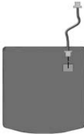
Figure 5-6. Disconnecting the Touch Button Cable
