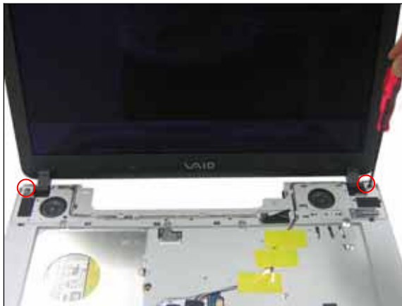
Step 17. Using a screwdriver remove the marked screw.
