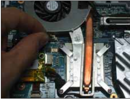
Step 29. Gently remove the ASSY Thermal CPU cable.
