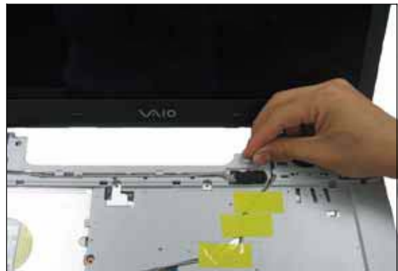
Step 16. Gently Pull out the LCD cable.
