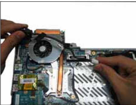
Step 31. Gently remove the DC IN cable.
