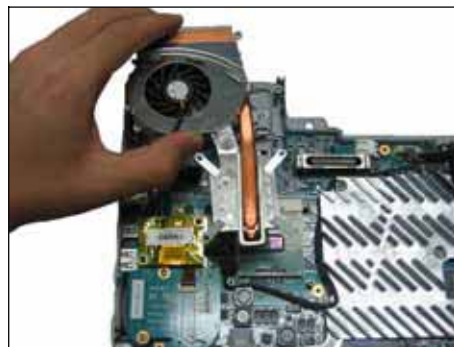
Step 32. Gently remove the ASSY Thermal CPU.
