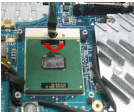
Step 33. Unlock the CPU socket as show.
