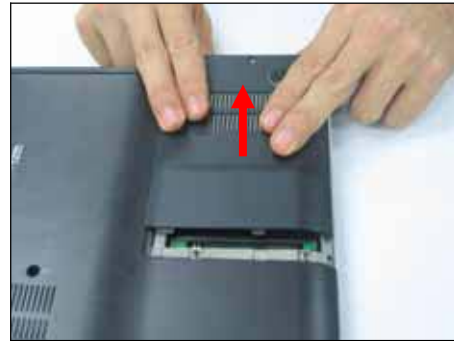
Step 6. Remove hard drive access door in the direction of the arrow and set aside.
