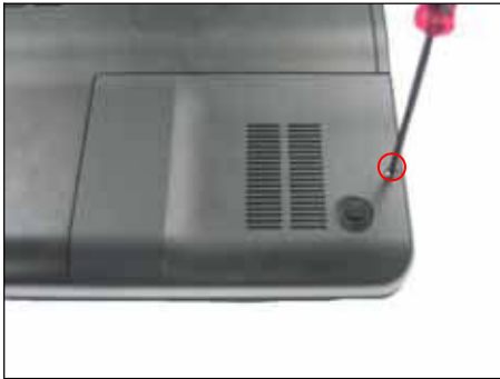
Step 5. Using a screwdriver, remove the marked screw .
