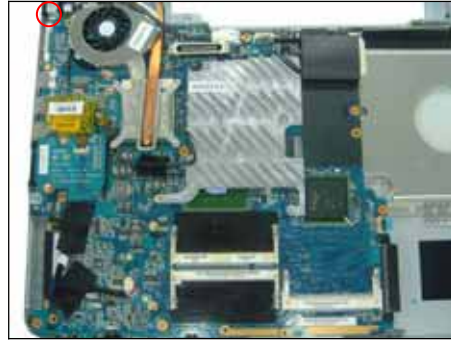
Step 30. Using a screwdriver remove the marked screw.
