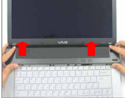
Step 10. Remove the KBCOVER in the direction of arrow and set aside.
