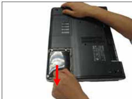
Step 8. Gently pull out HDD in the direction of the arrow and set aside.
