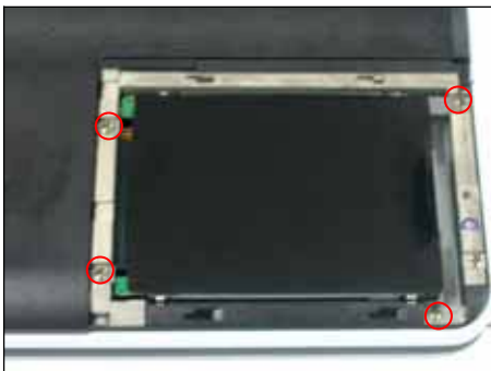
Step 7. Using a screwdriver remove the marked screw.
