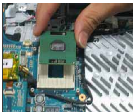
Step 34. Gently remove the CPU.
