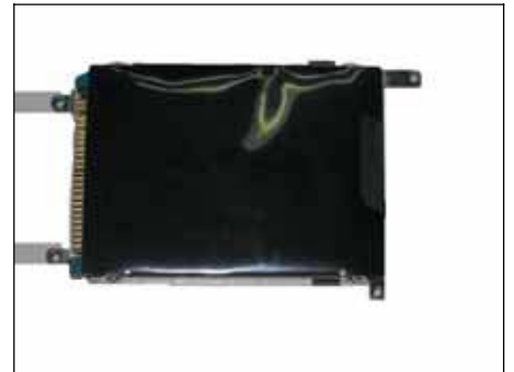
Step 8. Gently pull out HDD in the direction of the arrow and set aside.
