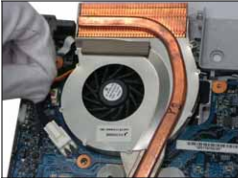
Step 30. Gently remove the ASSY Thermal CPU cable.
