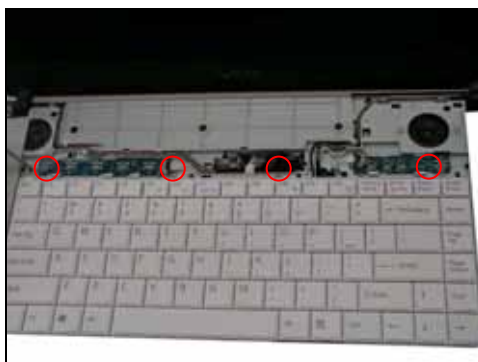
Step 13. Using a screwdriver remove the marked screw.
