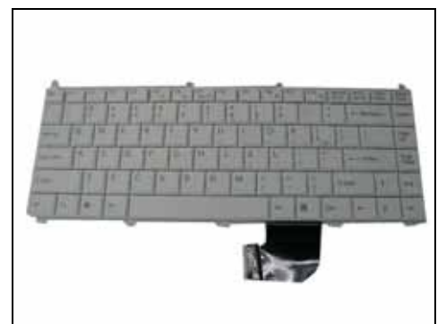
Step 14. Remove the keyboard data cable in the direction of arrow and set aside.
