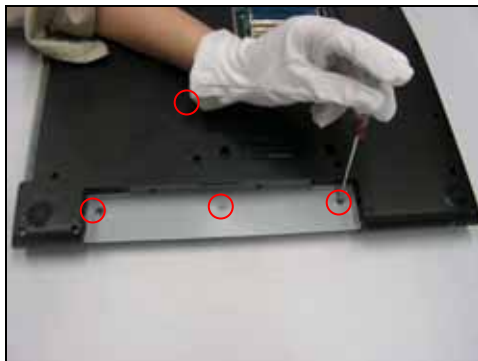
Step 11. Using a screwdriver, remove the marked screw.
