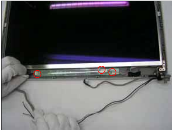
Step 20. Gently pull out the connector of the inverter as shown.
