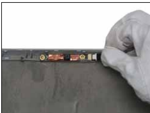
Step 23. Gently pull out the cable.
