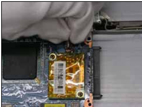
Step 34. Gently remove the Modem cable.
