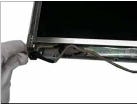
Step 22. Gently remove the Hinge and LCD panel.
