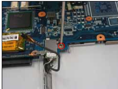
Step 35. Using a screwdriver remove the marked screw.
