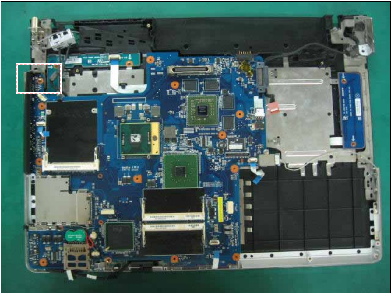
Step 57. Remove the Mother Board.
