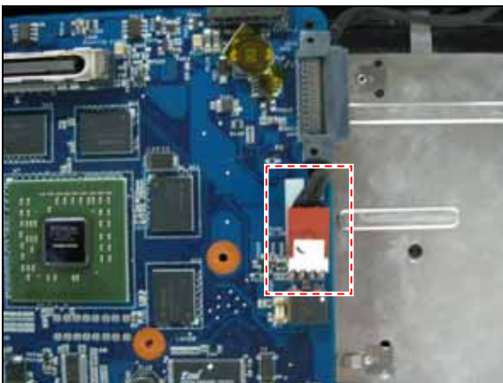
Step 55. Disconnect the DC JACK HARNESS.
