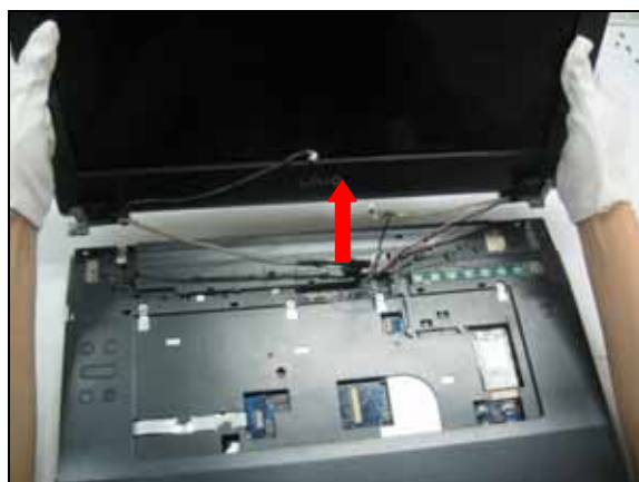
Step 18. Gently pull out the LCD.
