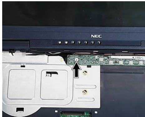
Fig. 10: Removing the LED's and switch board
