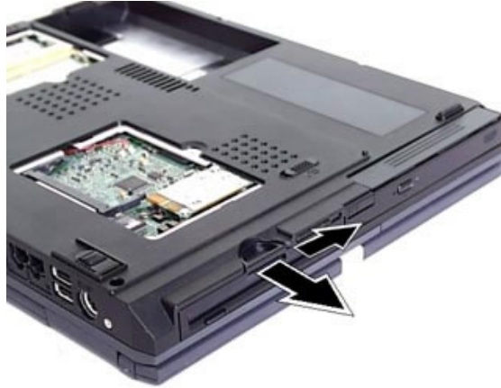
Fig. 5: Removing the floppy disk drive
