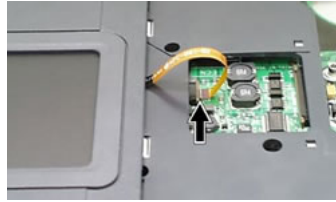
Fig. 22: Disconnecting the glide pad flat cable
