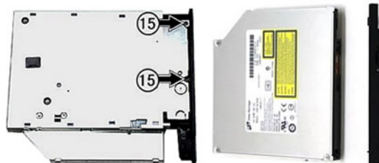
Fig. 58: Removing the front bezel
