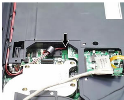
Fig. 17: Freeing up the wireless antenna wires
