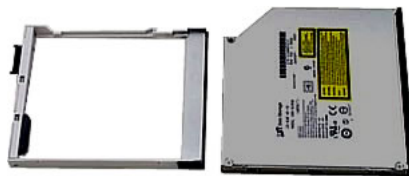
Fig. 56: Separating the optical drive from its frame
