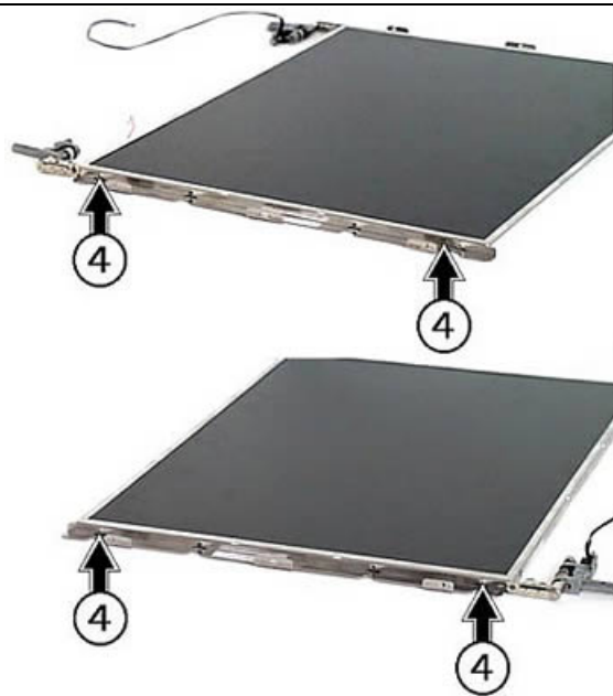
Fig. 52: Removing the LCD left and right hinges assembly
