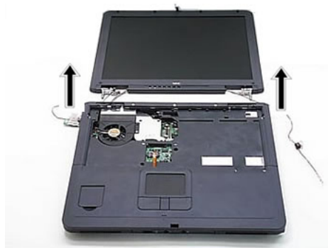
Fig. 21: Removing the LCD assembly
