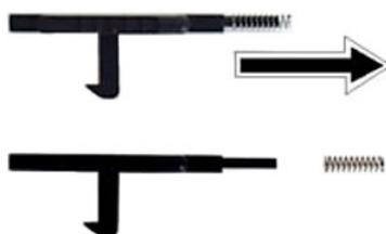
Fig. 47: Removing the latch spring
