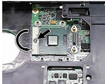
Fig. 14: Removing the CPU
