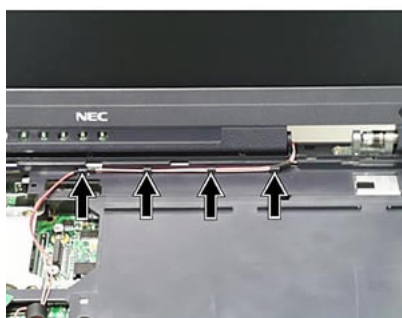
Fig. 18: Releasing the wireless antenna wires
