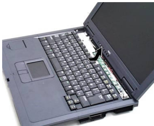
Fig. 8: Lifting up the keyboard
