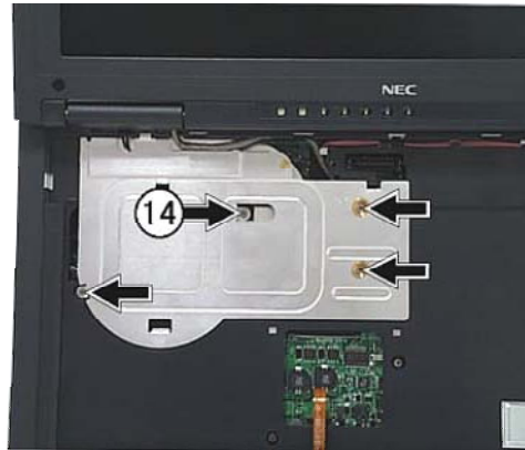
Fig. 11: Removing the thermal plate
