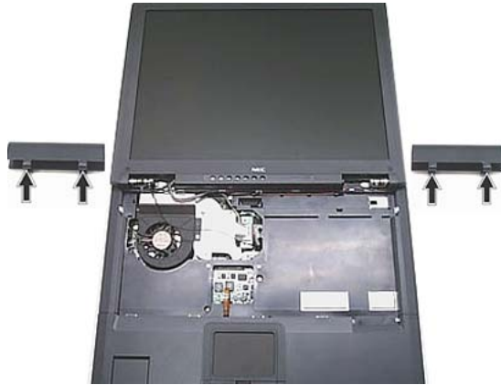
Fig. 15: Removing the plastic hinge covers
