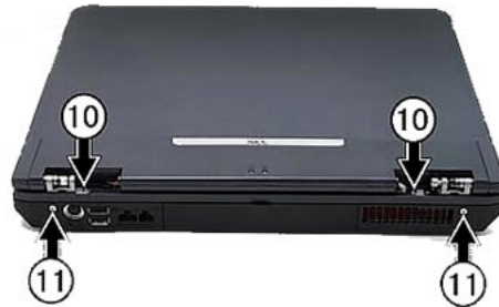
Fig. 20: Removing the 2 rear hinge screws
