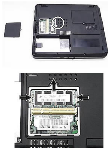
Fig. 2: Removing the memory module
