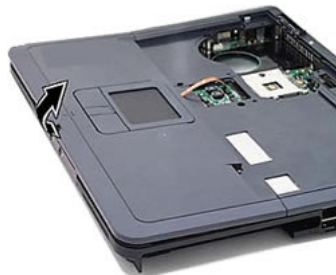
Fig. 24: Removing the glide pad assembly
