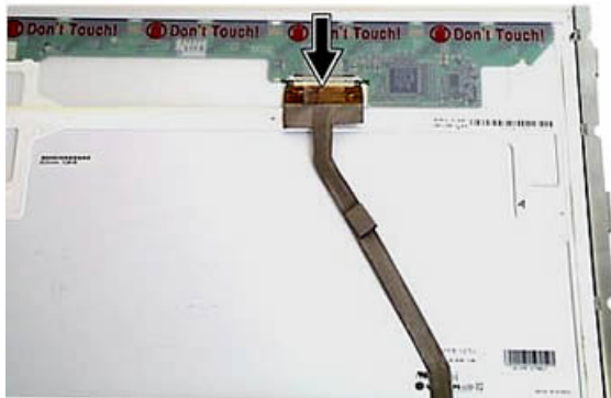
Fig. 51: Removing the LCD flat cable from the panel
