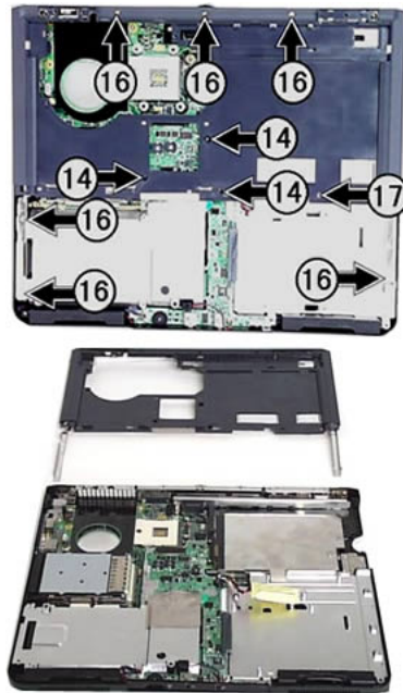
Fig. 30: Removing the plastic top cover
