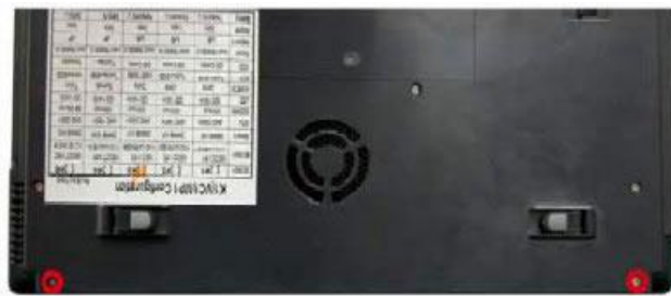
Fig. 13 Removing the LCD module screws (bottom).
