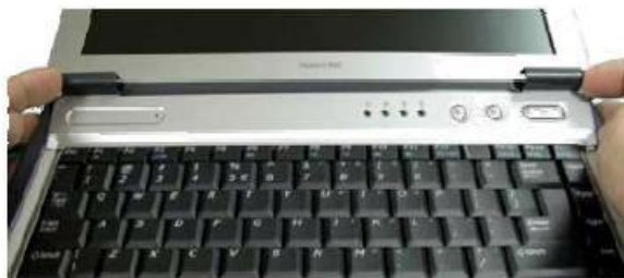
Fig. 7 Lifting the keyboard.
