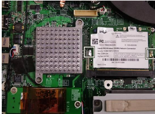
Fig. 27 Releasing the WLAN side locks.
