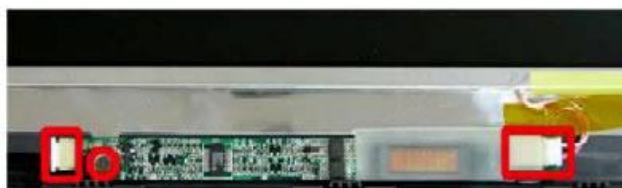
Fig. 17 Removing the inverter board.
