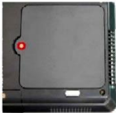
Fig. 2 Memory compartment cover screw location.
