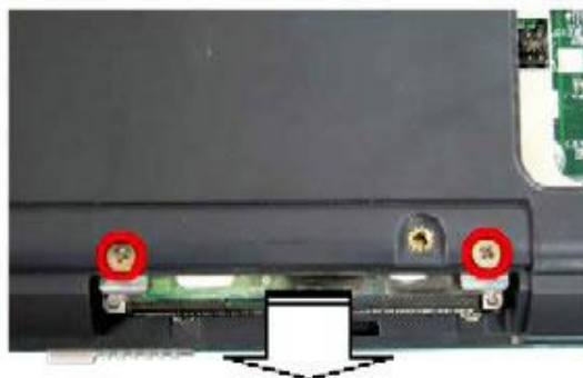
Fig. 5 Removing the HDD assembly.
