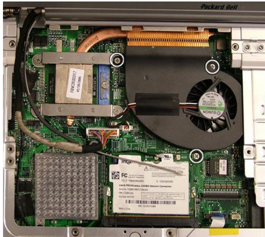
Fig. 19 Location CPU fan screws.
