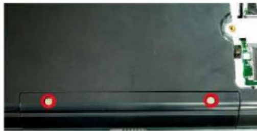
Fig. 4 Removing the hard disk drive cover.
