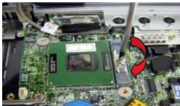
Fig. 21 Removing the CPU.
