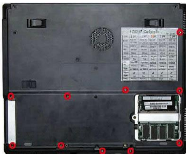
Fig. 22 Location bottom cover screws.
