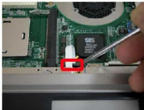
Fig. 24 Disconnecting the touchpad cable.
