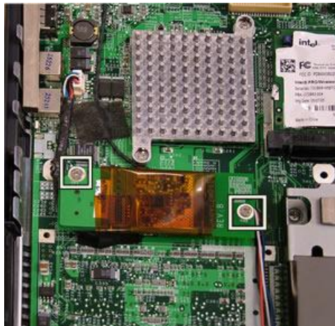
Fig. 28 Location modem card screws.
