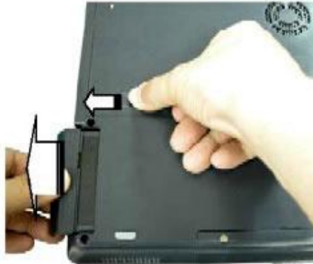
Fig. 1 Releasing the battery.
