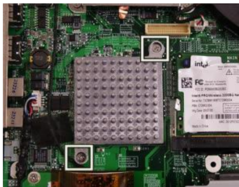
Fig. 26 Location chipset heat sink screws.
