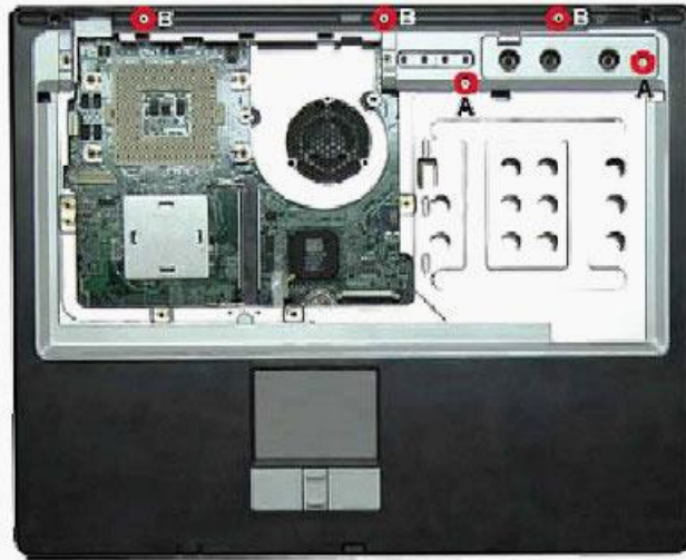
Fig. 23 Location top cover screws.
