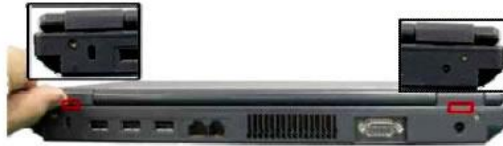
Fig. 6 Releasing the keyboard cover.
