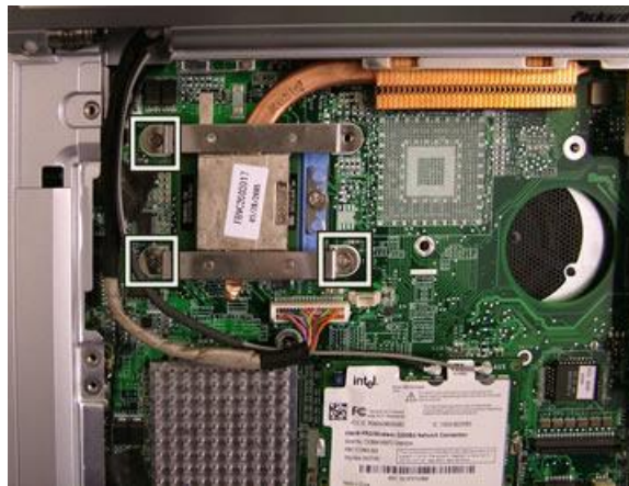
Fig. 20 Location remaining CPU heat sink screws.
