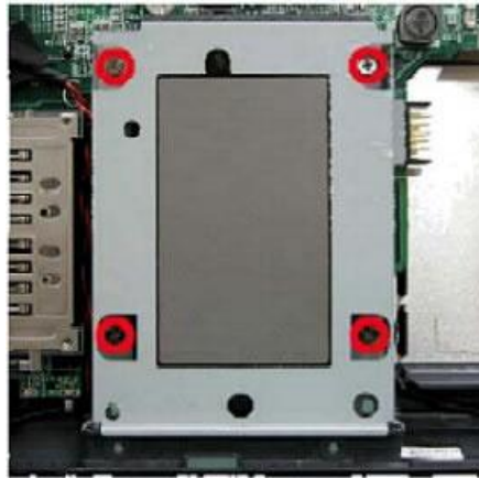
Fig. 29 Screw location on the HDD holder.
