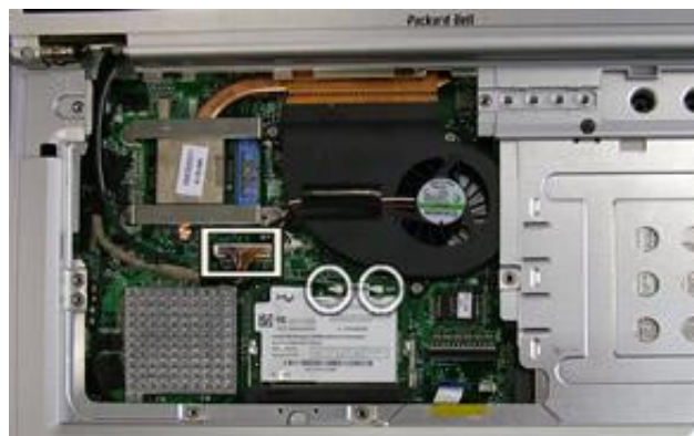
Fig. 15 Location WLAN antenna cables and LCD power cable.
