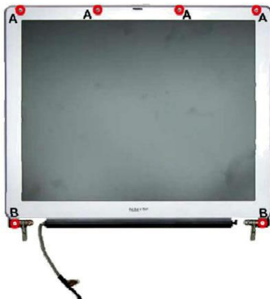
Fig. 16 Location of rubber covers and screws.
