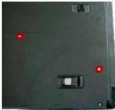
Fig. 10 Releasing the optical disk drive.
