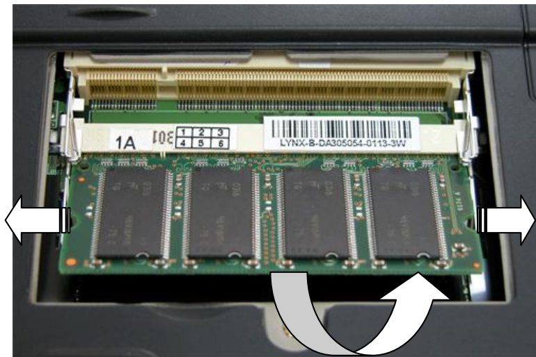
Fig. 7 Removing the memory module
