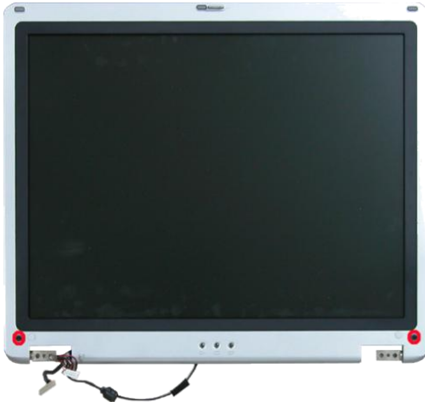
Fig. 27 Removing the rubber covers & screws on the LCD Module
