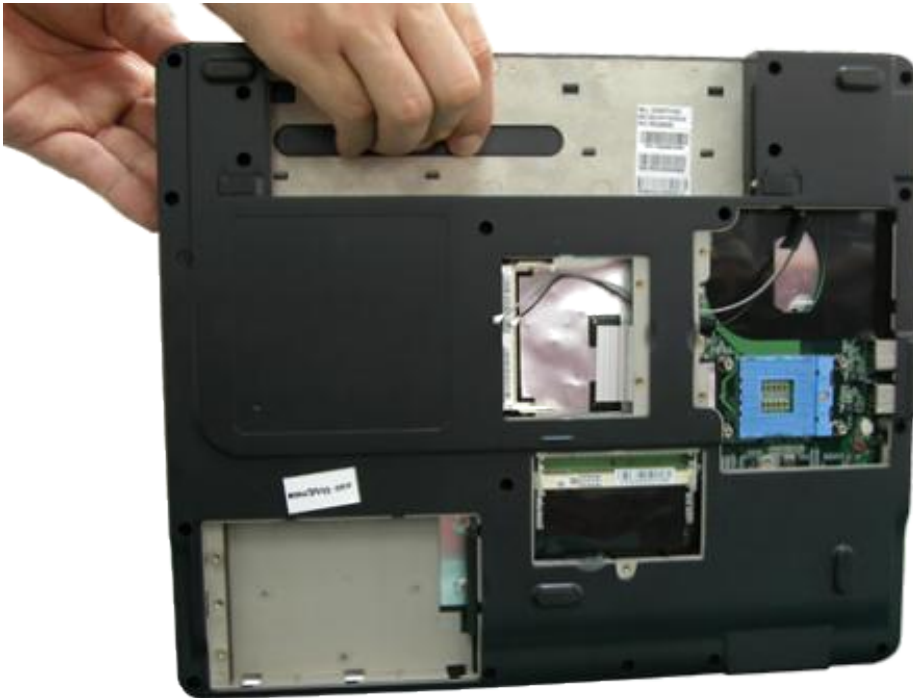
Fig. 16 Releasing the keyboard cover
