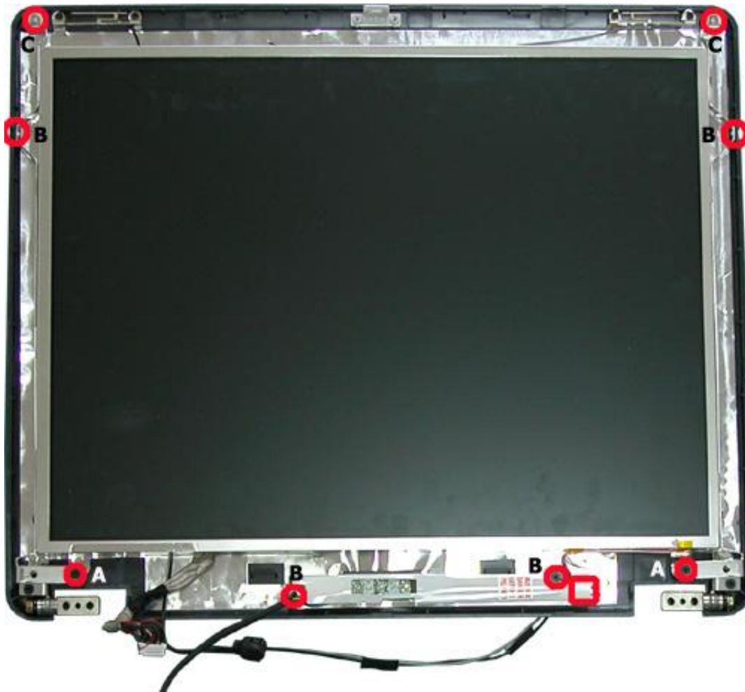
Fig. 29 Removing the LCD panel screws
