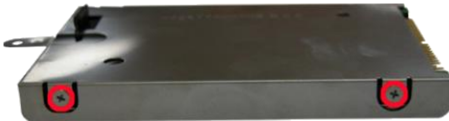
Fig. 5 Unscrewing the hard disk drive bracket screws
