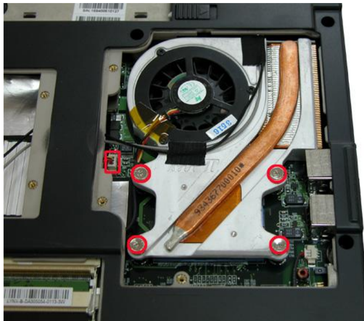
Fig. 11 Removing the screws retaining the heat plate. Exact location of CPU socket can differ from this image.
