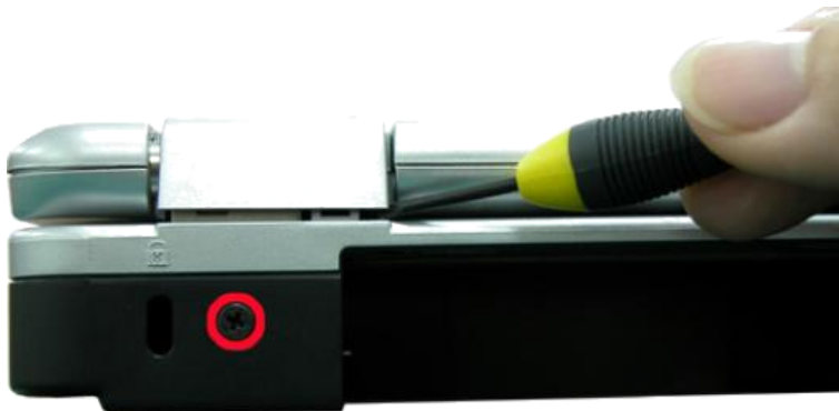
Fig. 19 Removing the top cover screws
