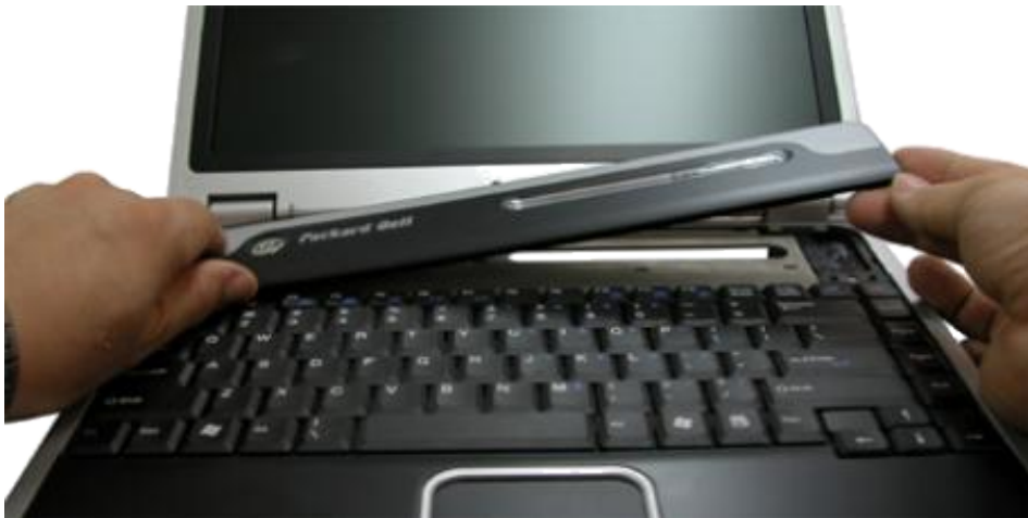
Fig. 17 Lifting up Keyboard Cover
