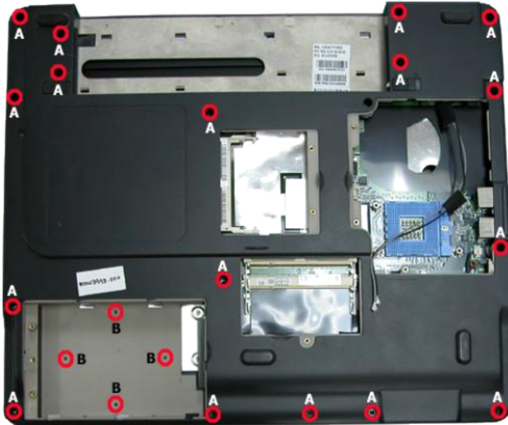
Fig. 22 Removing the top cover screws
