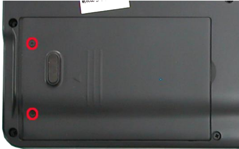
Fig. 2 Removing the Hard disk drive cover
