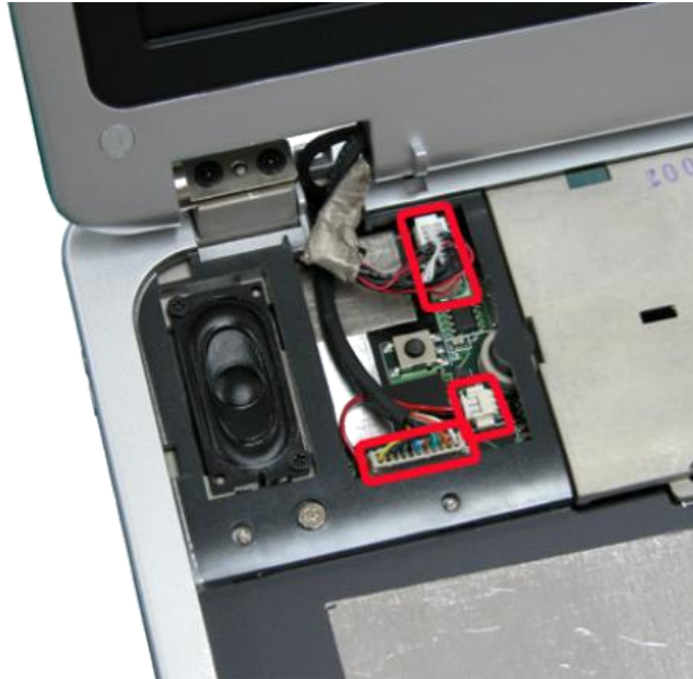
Fig. 20 LCD Cable and Left speaker connection
