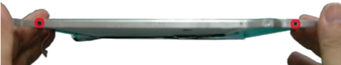
Fig. 30 Removing the LCD Panel hinges
