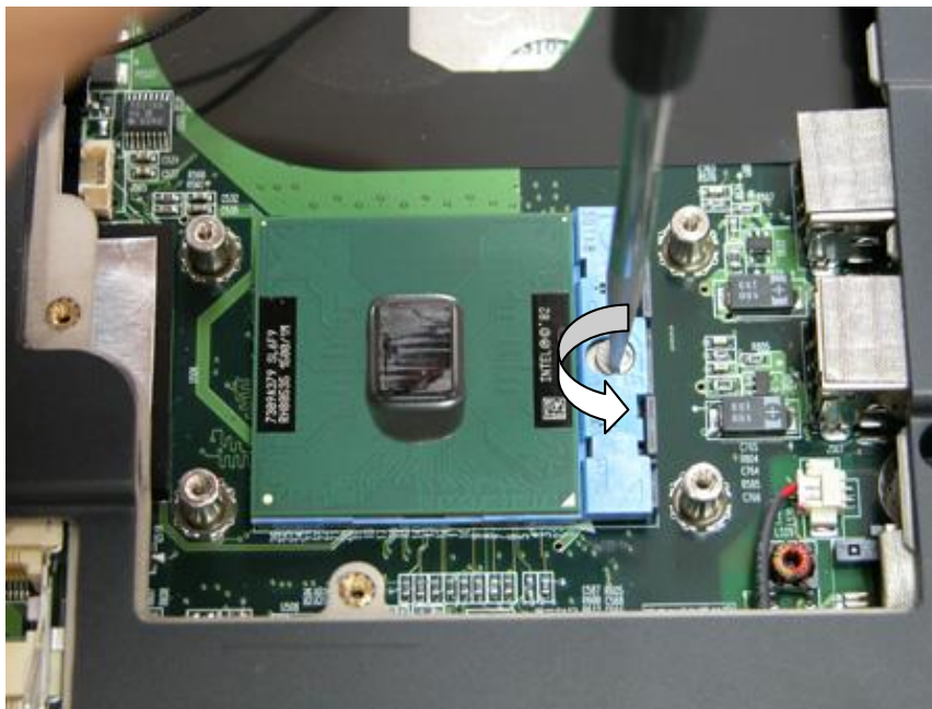
Fig. 12 Unlock CPU for EasyNote E2,E4 and E5.
