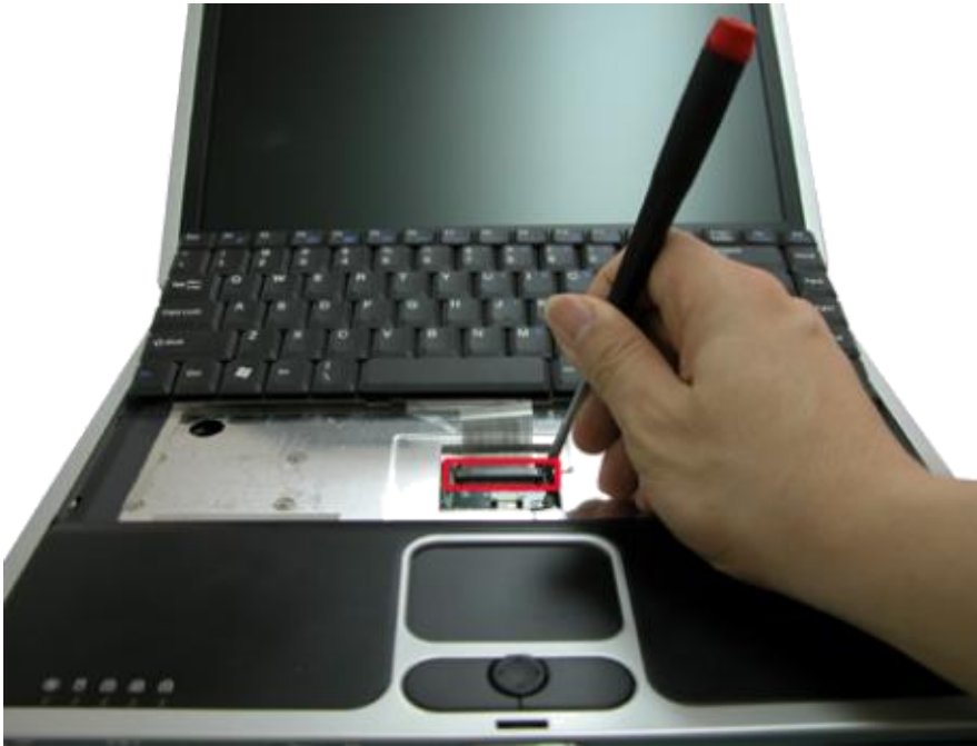
Fig. 18 Disconnect keyboard flat cable
