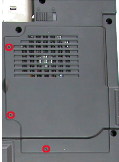
Fig. 10 Removing the screws retaining CPU cover
