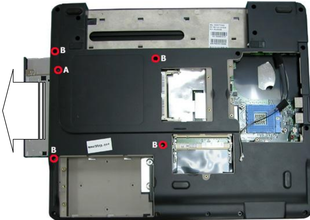
Fig. 15 Releasing the optical drive
