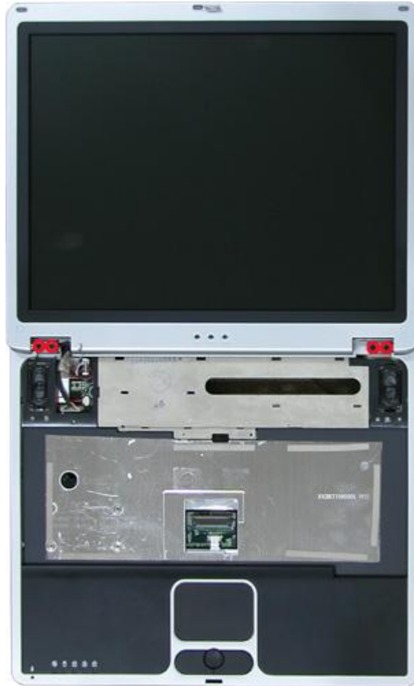
Fig. 26 Removing screws retaining LCD Module
