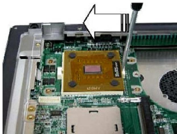
*Fig. 21 Unlocking the CPU*
