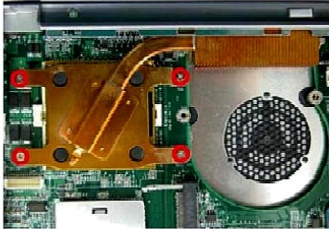
*Fig. 20 Removing the CPU heat sink screws*
