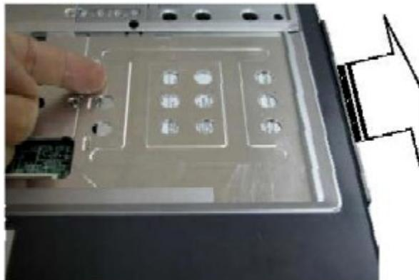
**Fig. 10** Pushing the optical drive out
