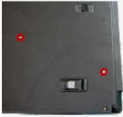
**Fig. 9** Releasing the optical disk drive
