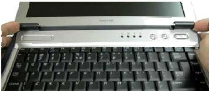
*Fig. 7 Lifting up the keyboard cover*
