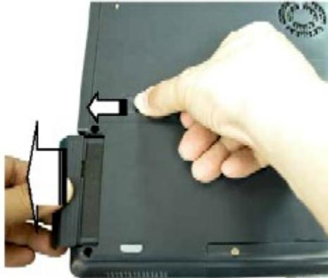
*Fig. 1 Releasing the battery*
