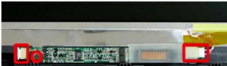
**Fig. 16** Removing the Inverter Board
