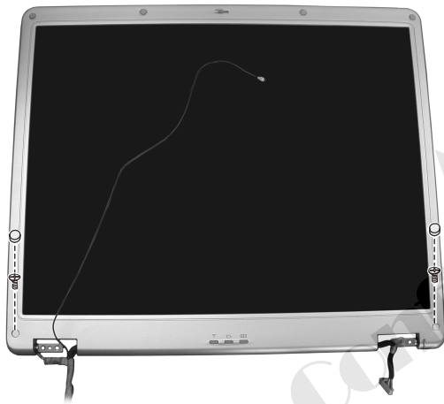
Figure 2-20 Remove LCD cover
