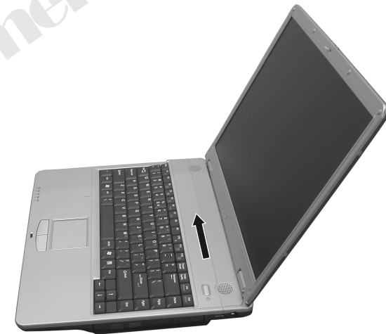
Figure 2-3 Lift the keyboard cover
