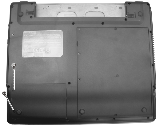
Figure 2-9 Remove the HDD compartment cover
