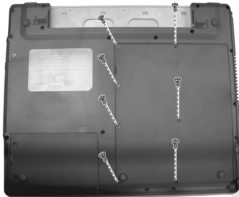
Figure 2-6 Remove the seven screws
