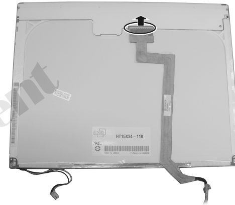
Figure 2-23 Free the LCD panel
