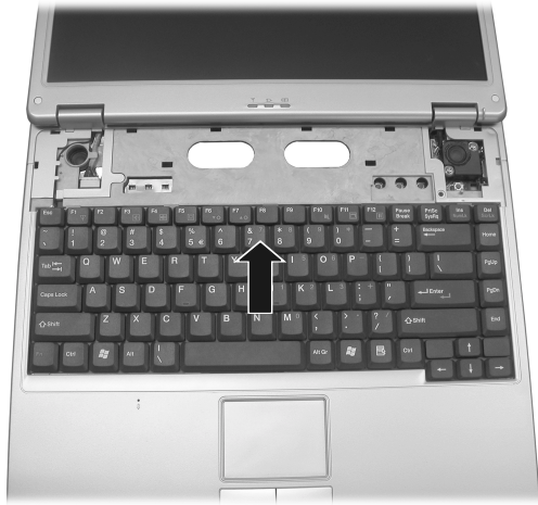
Figure 2-4 Lift the keyboard
