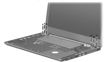
Where used: Two screws that secure the bezel to the display panel
