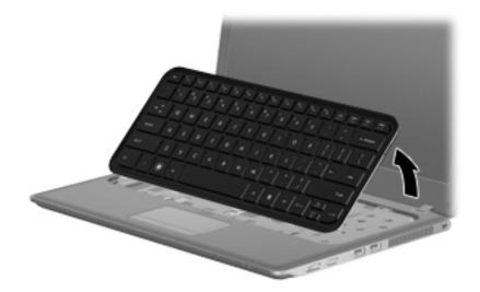
9. Carefully release the zero insertion force (ZIF) connector **1** to which the keyboard cable is attached, and then disconnect the keyboard cable **2** from the system board.
