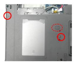
2. Put the screw driver here and push the ODD drive out from the NB.
