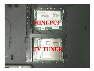
2. Disconnect the main Antenna and open the two latches to pop the MINI PCI MODULE up then pull it out.
