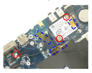
2. Remove 3 screws [M2 \* 4(W)] and take away the VGA thermal module.
