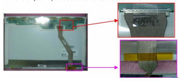
8. Remove 1 yellow tape and remove CCD module then disconnect the CCD cable.
