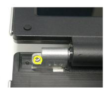
7. Remove 4 screws [M2.5  $^{\star}$  8(L)] on the Bottom case.
