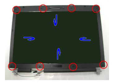
2. Carefully pry the inside edges of the LCD front bezel and remove the LCD front cover.
