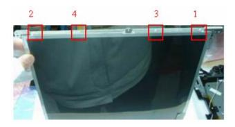
7. Remove 1 yellow tape and disconnect the coaxial cable from LCD.
