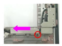
5. Remove 1 screw [M2 \* 4(L)] and remove the bracket then disconnect the cable and remove the Bluetooth board.
