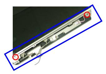
5. Remove 2 screws [M2 \* 5(L)] and remove the LCD module from the LCD back covert.
