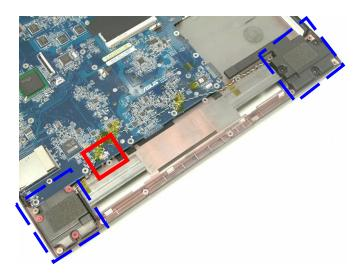
2. Remove 6 screws [M2 \* 6(L)] on the M/B.
