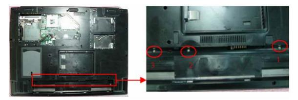
13. Remove 8 screws [M2 \* 4(L)] on the bottom case.
