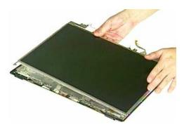
2. Finally, Remove 4 screws on the right LCD bracket, and 4 screws on the left side to disassemble LCD brackets.
