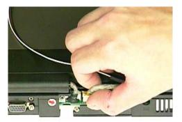
6. Remove 1 screw and disconnect the connector.
