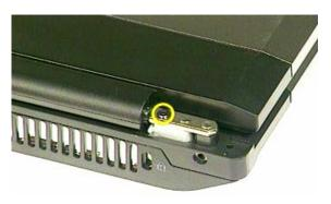
8. Remove the LCD module from system.
