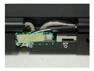
5. Remove 1 screw and disconnect the connector.
