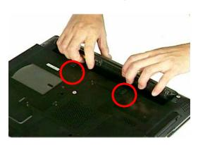
2. Slide the battery latch (No.1) to unlock and Firmly slide the other latch (No.2) to the top and remove the battery
