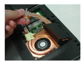
4. Turn the non-removable screw here 180 degrees counter-clockwise to loosen the CPU.
