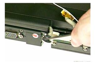
7. Remove 2 screws on both ends.
