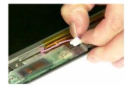
4. Disconnect inverter cable and take away the inverter board.
