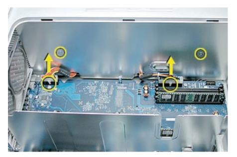
4. Remove the four power supply mounting screws on the bottom of the enclosure.
