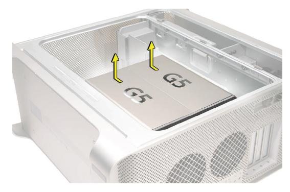
**Replacement Note:** Place the notches in the underside of the cover directly over the four mounting pegs. Slide the cover toward the back of the computer and then press down firmly until you feel the cover lock into place.
