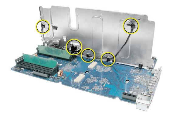
7. Turn the logic board over. Remove the three PCI divider mounting screws and remove the divider from the logic board.
