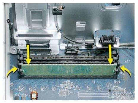
Important: Do not touch the DIMM connectors. Handle the DIMM only by the edges.
