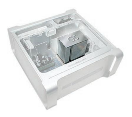
**Note:** The heatsink cover is held in place by two sets of small plastic latches on the underside of the cover.
