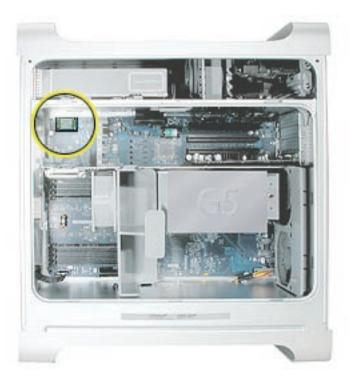
1. Remove the two Bluetooth mounting screws.
