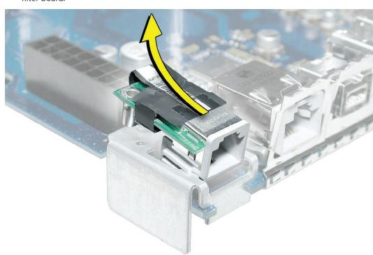
3. Slide the modem filter board off the metal frame to access another screw below the modem filter board.
