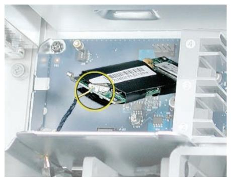
3. Remove the modem from the enclosure.
