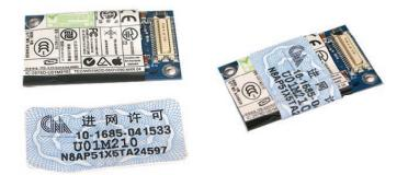
1. Connect the modem filter cable to the connector on the end of the modem board.
