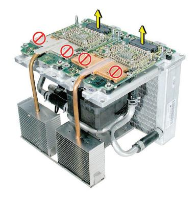
2. Loosen the screws marked below. **Delphi version**
