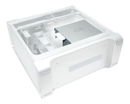
1. Tilt the processor inlet frame to the left and then up to unlatch the plastic piece from the heatsink.
