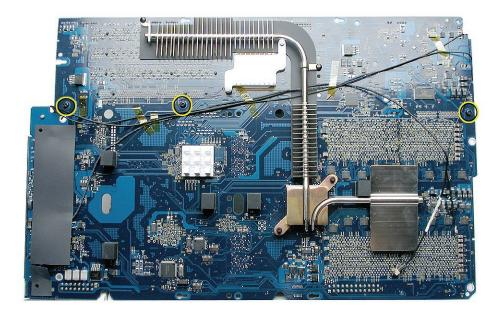
8. Position the PCI divider on the replacement logic board and install the three mounting screws.
