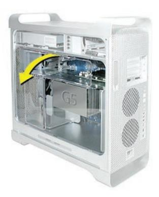
**Replacement Note:** To replace the air deflector, insert the three tabs on the bottom edge of the deflector into the three slots in the bottom frame of the enclosure. Then swing the deflector up flush against the top frame of the enclosure.
