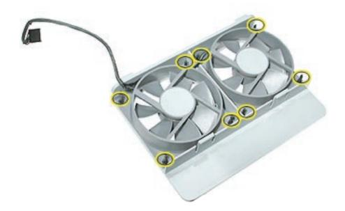
**Replacement Note:** When reinstalling the fan bracket in the enclosure, make sure the two tabs on the bottom of the bracket engage with the slots in the enclosure's fan guide.
