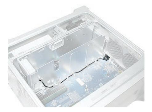
1. Disconnect the black antenna cable from the AirPort Extreme Card (if installed).
