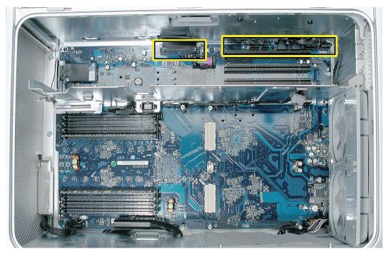
1. Disconnect the cables from the top of the logic board.
