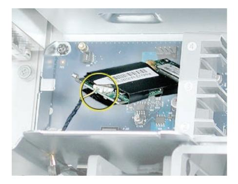
2. Connect the modem to the modem connector on the logic board and install the two mounting screws.
