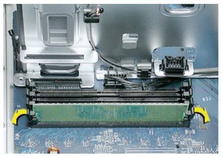
**Replacement Note:** Align the DIMM in the slot and push both ends of the DIMM down until the tabs are vertical and the ejectors snap into place.
