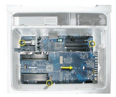
**Note:** When installing the logic board into the computer, make sure the antenna board shield is not bent back away from the case. The shield should touch the case when the logic board is fully installed.
