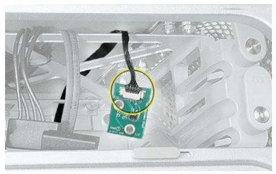
**Replacement Note:** Before installing the replacement board, apply the double-stick tape included in the sensor board kit to the back of the board. Then reconnect the media sensor board cable and press the board to the frame in the location illustrated below.
