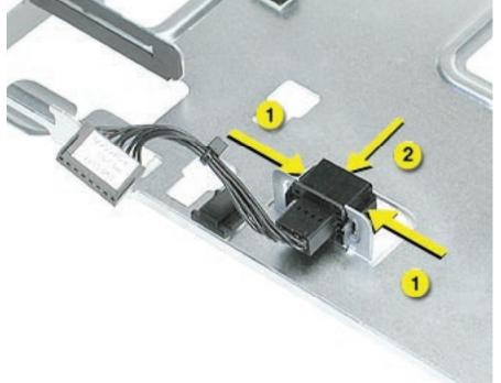
Remove the Bluetooth cable and AirPort cable from the cable guides on the PCI divider.
