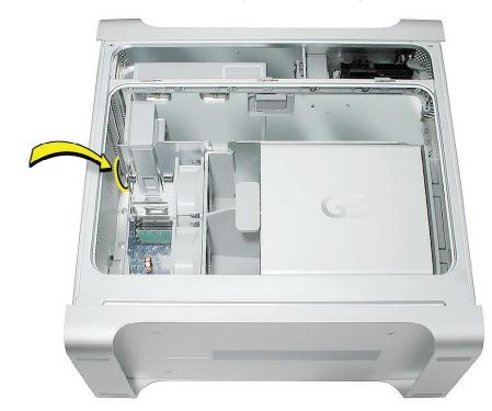
1. Locate the ambient board next to the speaker/fan assembly.
