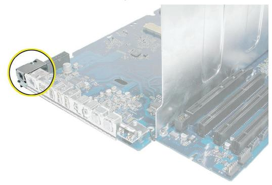
2. Remove the screw that secures the metal cover to the modem filter board. Remove the metal cover. Note: The cable routes under the logic board.
