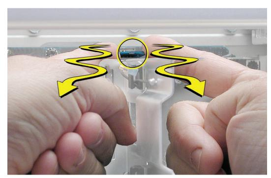
5. Position your fingers on both sides of the board. Gently rock the board from side-to-side, pulling it straight up and out of the connector.
