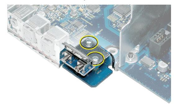
2. Remove the two antenna board mounting screws. Remove the board with the cables.
