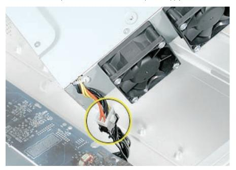
8. Remove the power supply from the enclosure.
