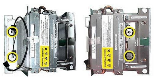
3. Check to make sure the top edges of both processors align.
