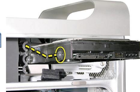
When installing a bottom drive, align the guide screws with the bottom slot of the drive bay and slide the drive in until it snaps into place.
