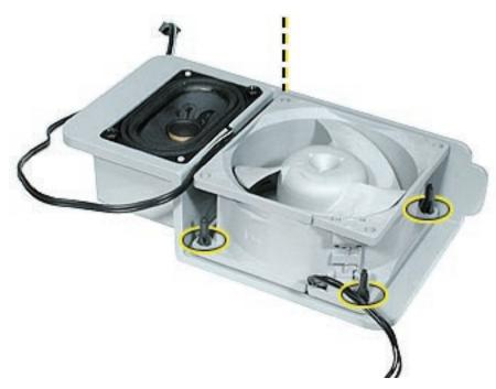
4. If you are replacing the fan, use needlenose pliers to pull the fan off the four grommet fasteners. Then remove the fan from the bracket.
