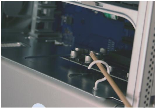
4. Slide the cover to the left to unlatch the four metal latches under the cover. Lift the cover up and off the heatsink.
