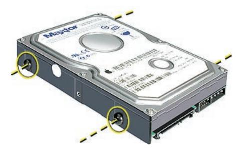
**Replacement Note:** When replacing the top drive, make sure the guide screws align with the middle slot of the drive bay, and then gently push the drive into the bay until it snaps into place.
