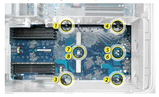
5. Lower the processor over the eight standoffs and two processor connectors.
