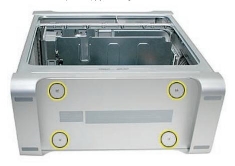
4. Remove the four power supply mounting screws on the bottom of the enclosure.
