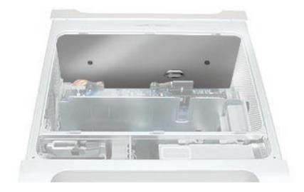
Remove the black plastic caps covering the two power supply cable connectors.
