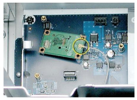
**Replacement Note:** Be very careful connecting the antenna cable to the Bluetooth card. The connector is fragile and can easily be bent.
