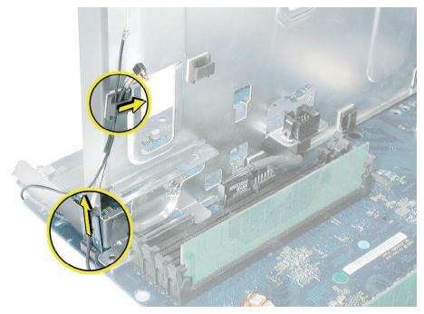
2. **Power Mac G5 (June 2004 Dual 2.5 GHz and Early 2005 Dual 2.7 GHz):** Remove the heatsink cable from the cable guides on the PCI divider.
