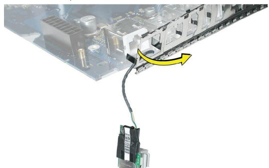
**Replacement Note:** If you replace the modem filter board, its cable (A below) routes underneath the logic board. (B=AirPort cable, C=Bluetooth cable)
