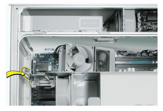
3. Set the speaker/fan assembly off to the side; there is no need to disconnect the assembly.
