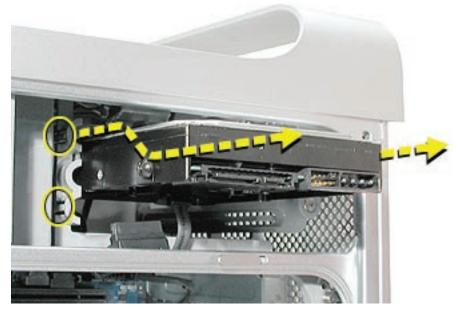
**Important:** If the printed circuit board (PCB) is exposed on the bottom of the hard drive, hold the drive by its sides. To avoid damaging the replacement drive, take care not to touch the PCB during installation.
