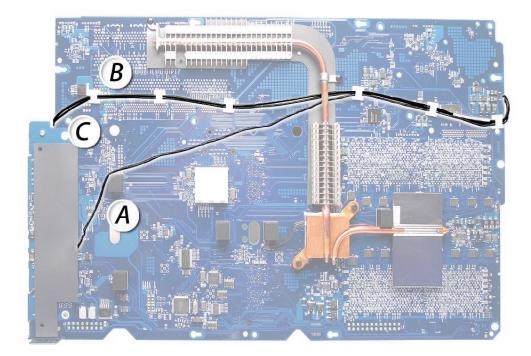
5. Pull the EMI fence away from the logic board just enough to free the modem filter board cable from the hole (see step 2) on the logic board. Note: The modem filter board, cable, and EMI are one service part.
