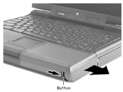
1 Push the button and slide the battery out of the media bay.
