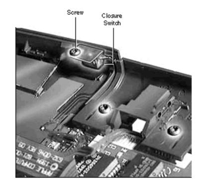
1 Remove the screw that holds the closure switch in place.
