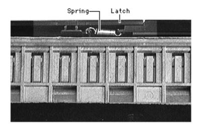
**Note** : It's a good idea to remove the latch any time you're working inside the display assembly. Removal allows the display to lay flat and evenly absorb any pressure exerted when screws are installed.
