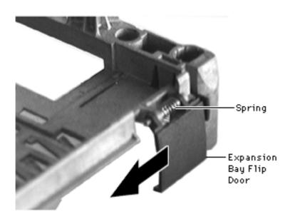
8 Slide the expansion bay flip door forward and gently remove the door and its spring.
