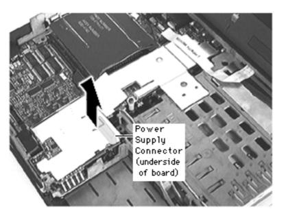
**Note:** The connector is located on the top right side of the power supply board.
