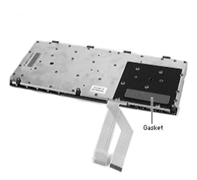
7 If a foam gasket is not already installed on the bottom of the keyboard, install a gasket (part number 922-3103) as illustrated.
