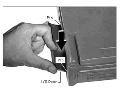
**Note** : The I/O door is held in place by 2 pins on the bottom case.
