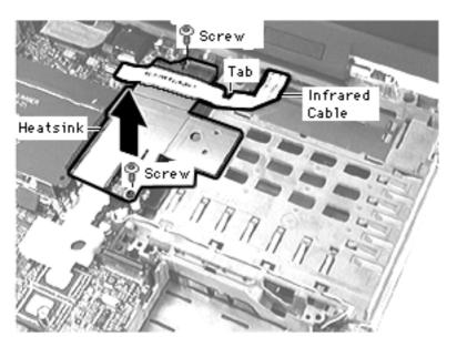
**Note:** The heat transfer sponge on the heatsink is tacky; keep it clean so it does not pick up dust from the workspace.
