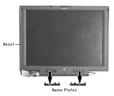
Using a plastic swizzle stick, remove the 2 product name plates from the bezel.
