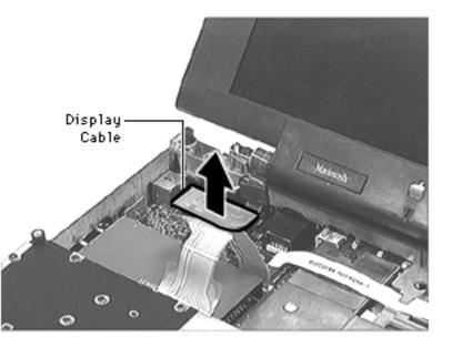
1 Gently disconnect the display cable from the logic board.
