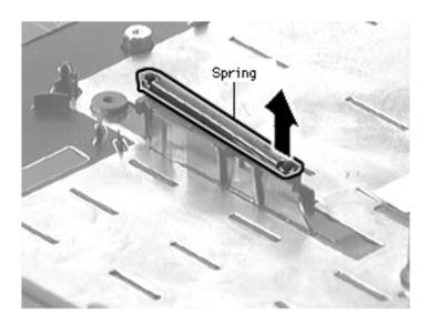
**Note** : The release mechanism assembly consists of a spring and plastic "hook and eye."
