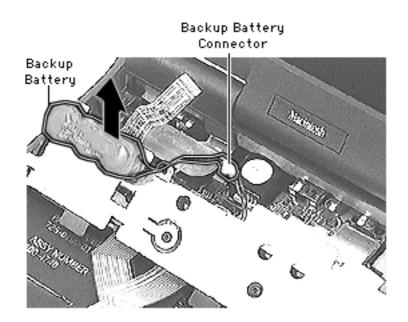
4 Using your fingers, disconnect the backup battery connector.
