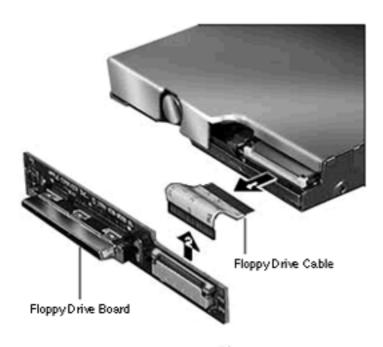
4 Using a dental pick, disconnect the floppy drive cable from the floppy drive and the floppy drive board.
