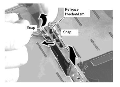
**Caution:** The following step, which frees the tightly installed release mechanism from the bottom case, is difficult to perform. Be careful not to break the plastic snaps.
