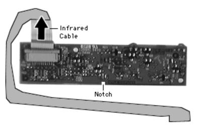
3 Disconnect the infrared cable from the board.
