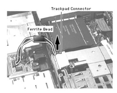
4 Using a dental pick, detach the trackpad connector.
