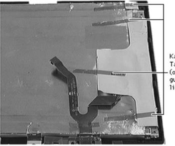
is only necessary to disconnect the display cable from the inverter board, not remove the inverter board. (Review the precaution for this step in the Inverter Board chapter.)
