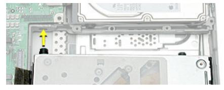
**Important:** When the rubber stoppers are inserted, push down on all four corners of the drive to verify that the drive is level and secure.
