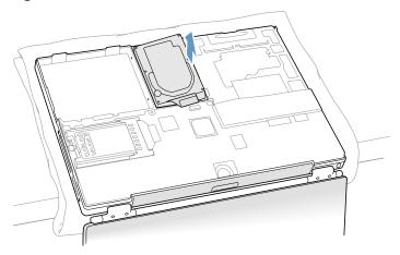
**Note:** There are four rubber stoppers on the hard drive that fit over screws (two on each side). Remove any that may have fallen off or that remain in the holes in the mounting bracket inside the computer.
