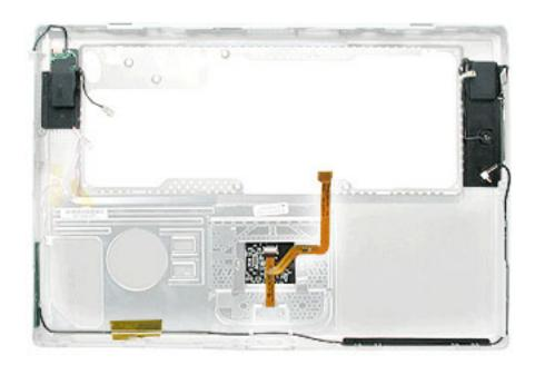
3. Important: Make sure you transfer the original serial number label from the old top case to the serial number panel on the replacement top case. You can use a black stick or razor blade to carefully peel up a corner of the label. Then peel off the label completely and apply it to the serial number panel. Make sure that the label lies completely flat so it does not interfere with the battery compartment.
