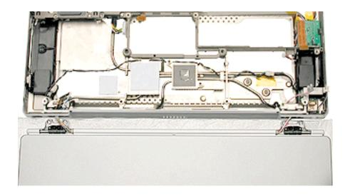
13. Remove the four rib frame screws. Three are identical black T8 screws, the forth is a longer chrome T8 and also secures the heat exchanger alignment bracket to the end of the heat exchanger. (You might need to move aside the AirPort antenna cable to reach one of the screws.)
