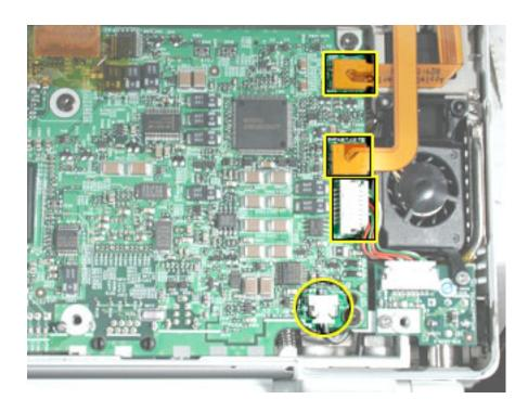
7. Disconnect the trackpad, hard drive and optical drive flex cable connectors.
