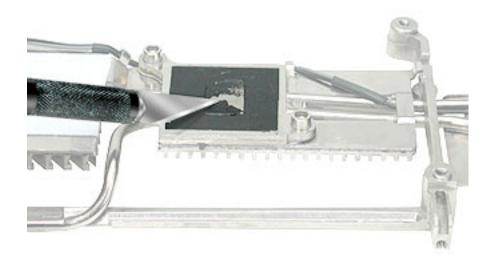
**Replacement Notes:** If replacing the heat exchanger, transfer the hex nut and screw to the replacement heat exchanger.
