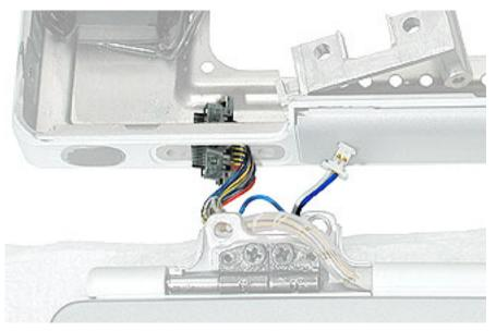
4. At the right clutch, raise the inner clutch mount and disconnect the inverter cable. Carefully slide the inverter cable out through the opening in the top case.
