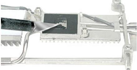
17. Important: If you have removed the logic board to access another part, and you will be placing the original logic board back in the computer, use a black stick to gently scrape away any residual thermal transfer material from the microprocessor chip on the logic board.
