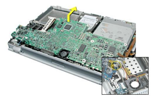
**Replacement Note:** When reassembling the computer, make sure the replacement logic board ports align completely with the openings in the back panel.
