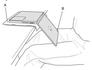
6. Remove the battery by sliding the battery latch to the left. Make sure to return the latch fully to the right. (Figure 2)
