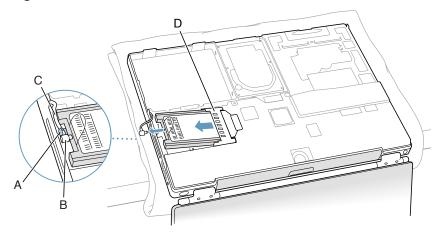
**Important:** If reassembling the computer without an AirPort Card, replace the antenna cable connector into its holder (**Figure 9B**) and pull the loop of the antenna cable up slightly and away from the edge of the computer case. This prevents the cable from interfering with the PC card slot, below, or getting pinched during reassembly.
