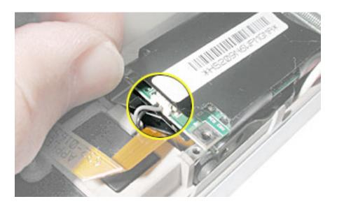
9. Use a thin tool to lift the optical drive slightly, then deroute the modern flex cable.
