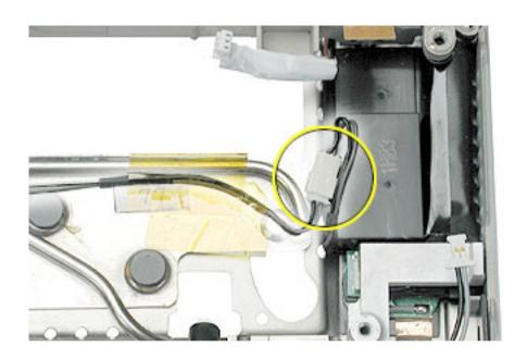
16. Pivot the heat exchanger out of the top case assembly. Be careful where it might catch at the LVDS cable.
