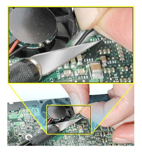
3. Turn over the logic board, then tilt up the fan to remove it completely from the logic board.
