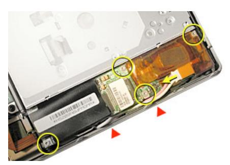
8. Lift up the end of the modem slightly and disconnect the 2-pin cable connector.
