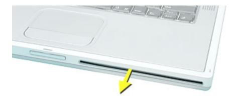
**Important:** Check the operation of the optical drive. If the drive is installed incorrectly, the optical drive mechanism might not spin correctly and will result in mechanical noise when playing a disc.
