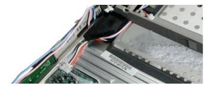
6. Install the replacement top case, and reassemble and test the computer.
