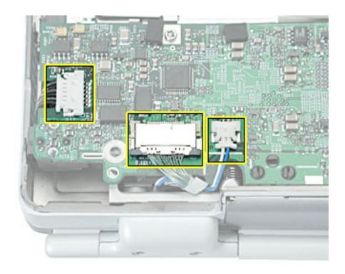
6. At the right side of the logic board, disconnect the 2-pin power button cable connector, the DC-in board cable connector, and the inverter board and modem flex cable connectors.
