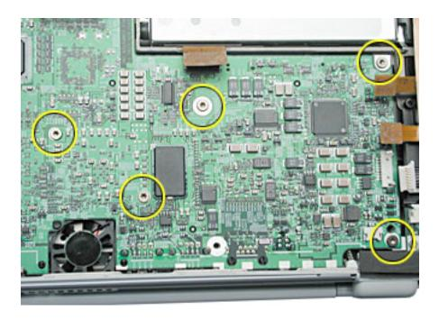
11. Grasp the logic board near the AirPort Card carrier and gently lift the board up, as shown below, being careful where it catches on ports, back panel mesh liner, and disconnected cables.
