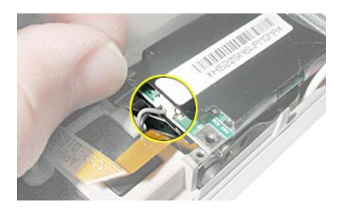
8. Use a thin tool to lift the optical drive slightly, then deroute the modern flex cable.
