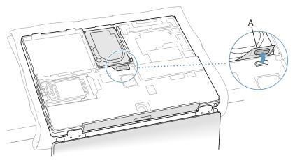
2. With a Torx T8 screwdriver, remove the two screws that secure the hard drive mounting bracket, and remove the bracket. (**Figure 8**)
