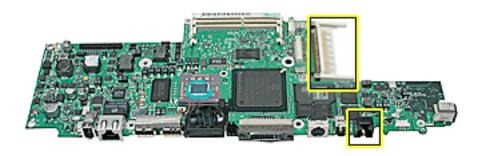
• U-shaped EMI clip between the FireWire and Ethernet ports
