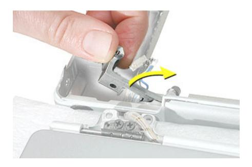
3. Thread the 2-pin LED sleep cable through the opening in the top case.
