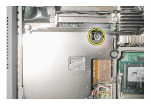
2. Disconnect the PC card flex cable connector and the keyed battery connector.
