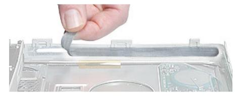
Apply the new felt strip to the slot-load area. Make sure the new felt strip lies flat. Use a black stick to run the length of the slot to make sure that the felt strip does not block any of the slot.
