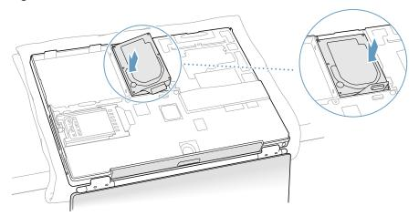
Replace the hard drive mounting bracket and secure with the screws. (Figure 12)
