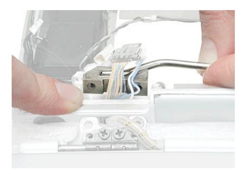
17. If replacing the rib frame but reusing the heat exchanger, scrape off the thermal transfer material residue from the area shown. Apply new thermal transfer material to the logic board chip.
