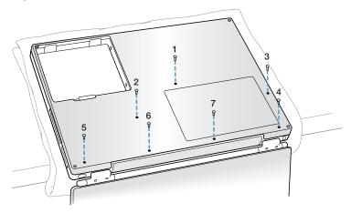
**Note:** In the following two steps you will disengage the left and right sides of the bottom case and then pivot it forward to remove.
