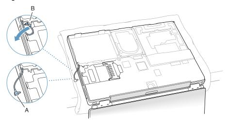
Position the AirPort Card (Figure 10B) with the AirPort ID numbers and bar code facing up. Pull up the insertion end of the AirPort Card connector (Figure 10A) slightly and slide the card all the way into the connector until it is securely attached.
