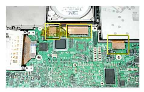
8. Remove the T8 screw on the edge of the logic board near the battery well.
