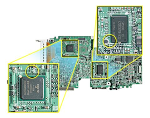
Plastic 1 mm and 1.5 mm washers around the screw holes, shown. Center and press into place.
