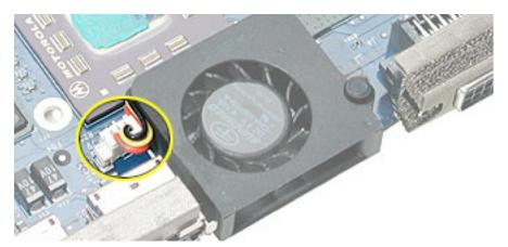
2. Turn over the logic board, and locate the cone-shaped pin at the right corner of the fan. Pull the rubber pin tight. Use a razor blade to cut through the rubber pin.
