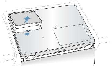
7. Use a Torx T8 screwdriver to remove the seven bottom case screws in the order shown. (Figure 3)
