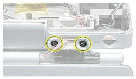
12. **Important:** With the display hinge disconnected, support the display as you place it face-down on a soft cloth in front of the computer chassis.
