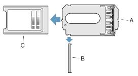
If necessary, pull the AirPort antenna cable connector (Figure 9A) from its holder (Figure 9B).
