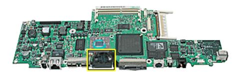
• EMI gaskets to the USB ports, FireWire port, DVI-I port, and headphone port, (use an I/O EMI gasket kit)
