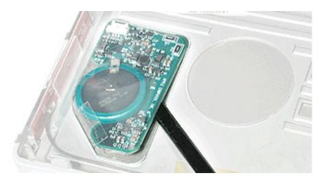
3. If there is any adhesive left on the surface of the inner top case, use a black stick to rub it away. Do not use solvents.
