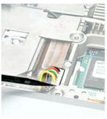
**Replacement Note:** When reassembling the computer, tuck down the battery cables so they do not get in the way when the keyboard is installed.
