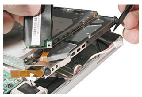
10. Warning: To prevent damage to the optical drive, handle the drive only by the corners. Do not press on the body of the drive.
