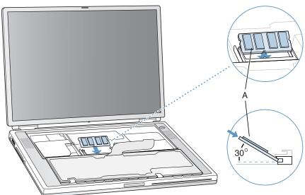
2. Gently push the card down until the two brackets on either side of the card lock into place (**Figure 8**).
