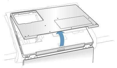
10. Touch the computer's inside framework (a dull gray conductive composite material) to discharge any static electricity, as shown. (Figure 6)
