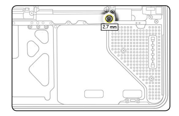
**2** Lift out battery cable guide.
