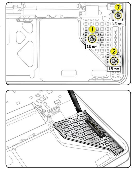
**2** Lift out battery connector cover.
