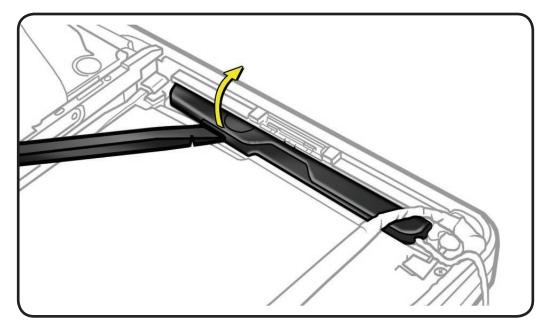
**2** Pry up speaker body to loosen adhesive.
