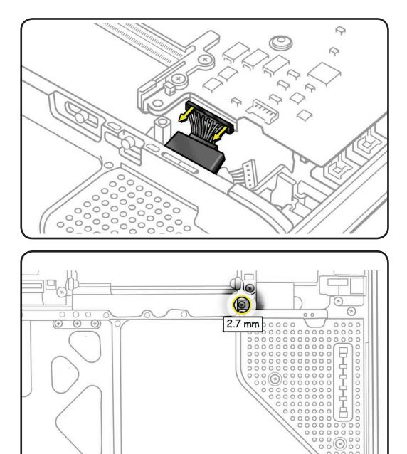
If necessary, remove 2.7-mm screw (922-8661) and battery cable guide to disconnect battery connector.
