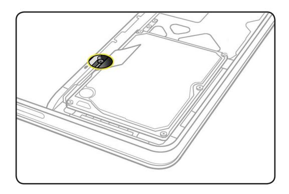
**2** Lift out retaining bar.
