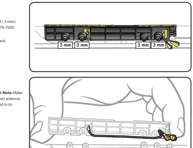
Replacement Note: Make sure the AirPort antenna cable is routed in its channel.
