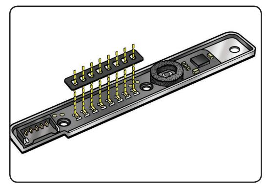
**3** Press cable so it lays completely flat.
