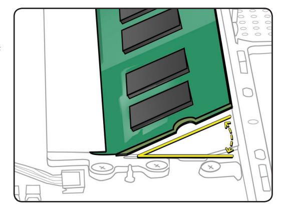
**2** Spread ejection levers, and press card down.
