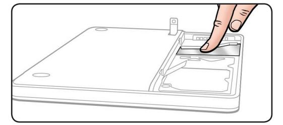
2 Make sure 4 rubber grommets are included in top case before installing the hard drive.
