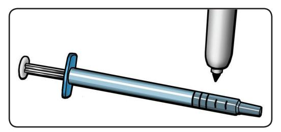
**2** Inject 1/3 of grease on each microprocessor.
