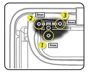
2 Use a black stick to tilt out the camera cable guide.
