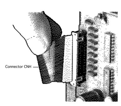
Disconnect connector CNH from the logic board.
