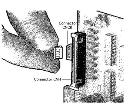
Disconnect connectors CNH and CNCR from the main board.
