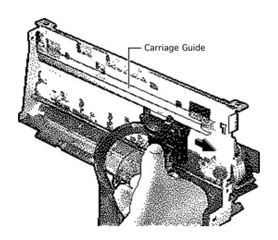
Move the carriage to the far right and disconnect the carriage from the carriage guide.
