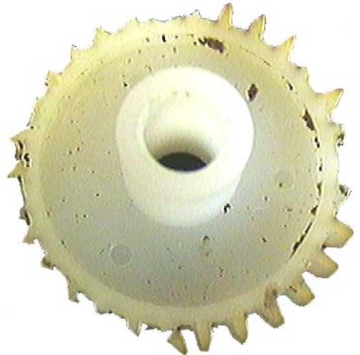
Original 'Q' Gear w/damaged teeth
