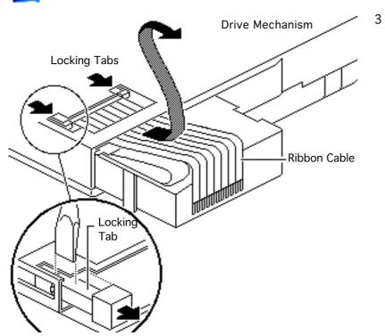
Using a jeweler's screwdriver, release the locking tabs and remove the ribbon cable from the drive.
