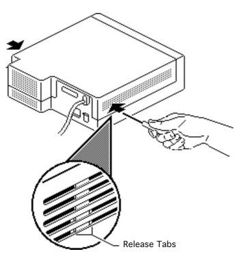
2 Using a jeweler's screwdriver, release the tabs that hold the cover.
