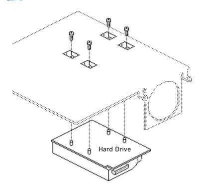
2 Remove the four mounting screws and the hard drive.
