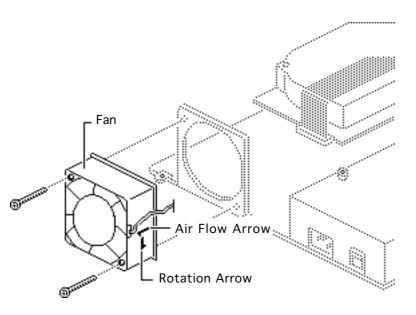
Remove the two mounting screws and the fan.
