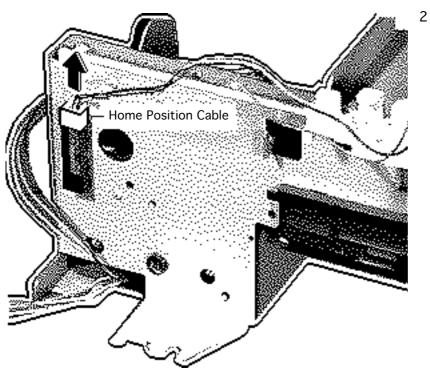
Disconnect the home position cable from the photo interrupter.
