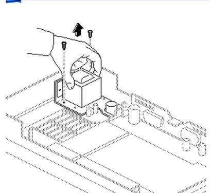
7 Remove the two remaining screws and lift out the transformer.
