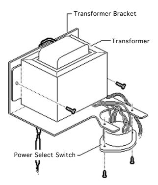
On universal transformers only, remove the two mounting screws and separate the power select switch from the transformer bracket.
