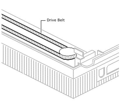
**Note:** You do not have to remove the drive belt from the optical block.
