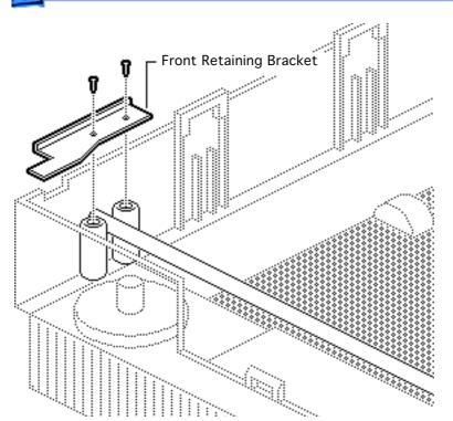
10 Remove the two retaining screws and the carrier shaft front retaining bracket.
