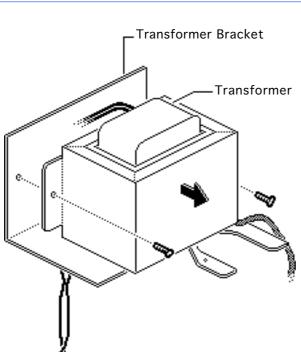
8 Remove the two mounting screws and separate the transformer from the transformer bracket.
