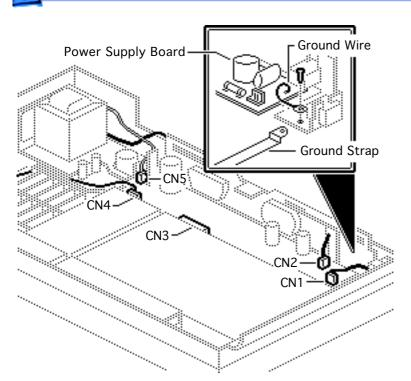
Replacement Note: A new power supply board includes the grounding strap. Loosen the grounding screw on the new power supply board, carefully move the grounding strap, and install the board and strap in the scanner.
