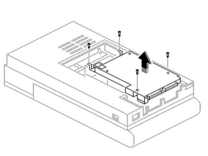
Remove the four mounting screws, and remove the logic board.
