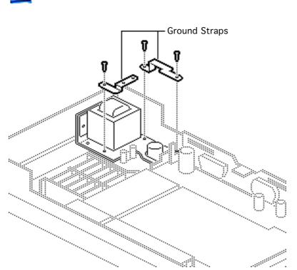
6 Remove the three screws and two ground straps.
