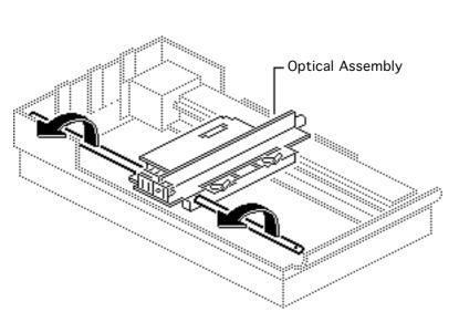
11 **Caution:** Do not lift the optical assembly too high, or you may damage the flex cable.
