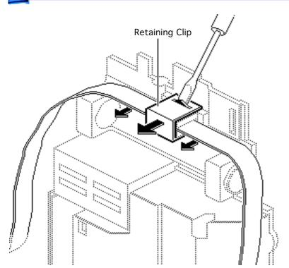
17 Using a small screwdriver, pry off the retaining clip and remove the belt from the optical assembly.
