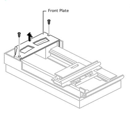
Remove the two retaining screws and lift out the front plate.
