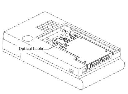
Caution: Do not let the optical cable slide back into the scanner. Tape it to the chassis until you can reinstall the logic board.
