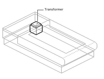
To convert a 110 V scanner (without the universal voltage selector) to a universal model, remove the transformer and bracket plate assembly and install the universal model transformer and bracket plate assembly.
