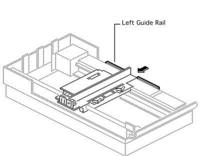
4 Push the optical assembly to the center over the cutout in the left guide rail.
