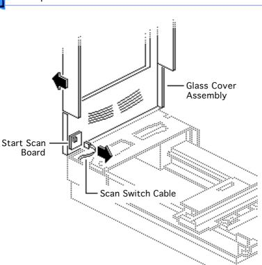
Caution: When removing the glass cover assembly, make sure you don't damage the start scan board.
