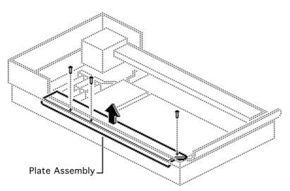
1 Remove the three mounting screws and lift out the plate assembly.
