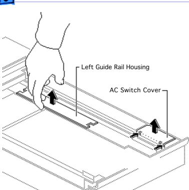
Note: To access fuses FU2 and FU3, lift the center of the left guide rail housing and remove it from the left guide rail.
