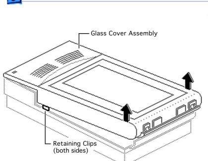
2 Lift the glass cover assembly from the rear, and at the same time press in and release the two retaining clips.
