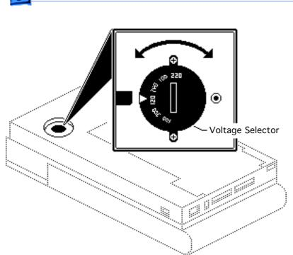
2 Using a coin or a flatblade screwdriver, rotate the voltage selector to match the incoming voltage.
