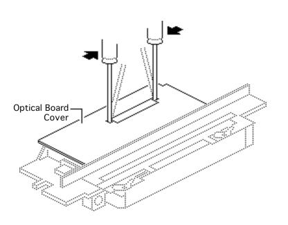
Using a flat-blade screwdriver unlatch the optical board cover.
