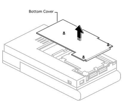
Loosen the three captive screws and remove the bottom cover.
