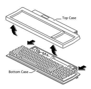
Grasp the bottom and top of the case. Push in on the tabs and lift off the top cover.
