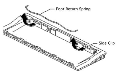
Pull the keyboard assembly toward the back of the bottom case to separate it from the front foot.
