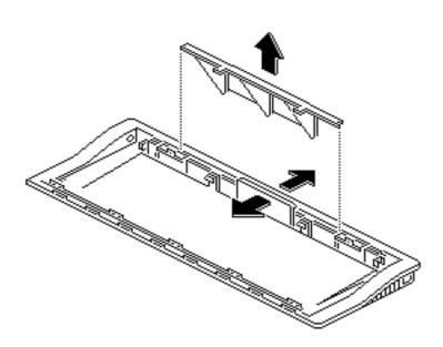
Spread the plastic clips and pull the height adjustment lever up and out.
