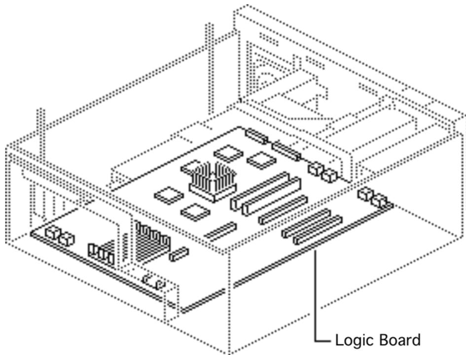
**Important:** You must install the processor fan with the WS 9150/120 logic board or you will damage the board.
