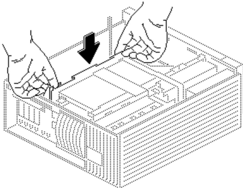
Gently push down on each end of the card to install it in the NuBus slot.
