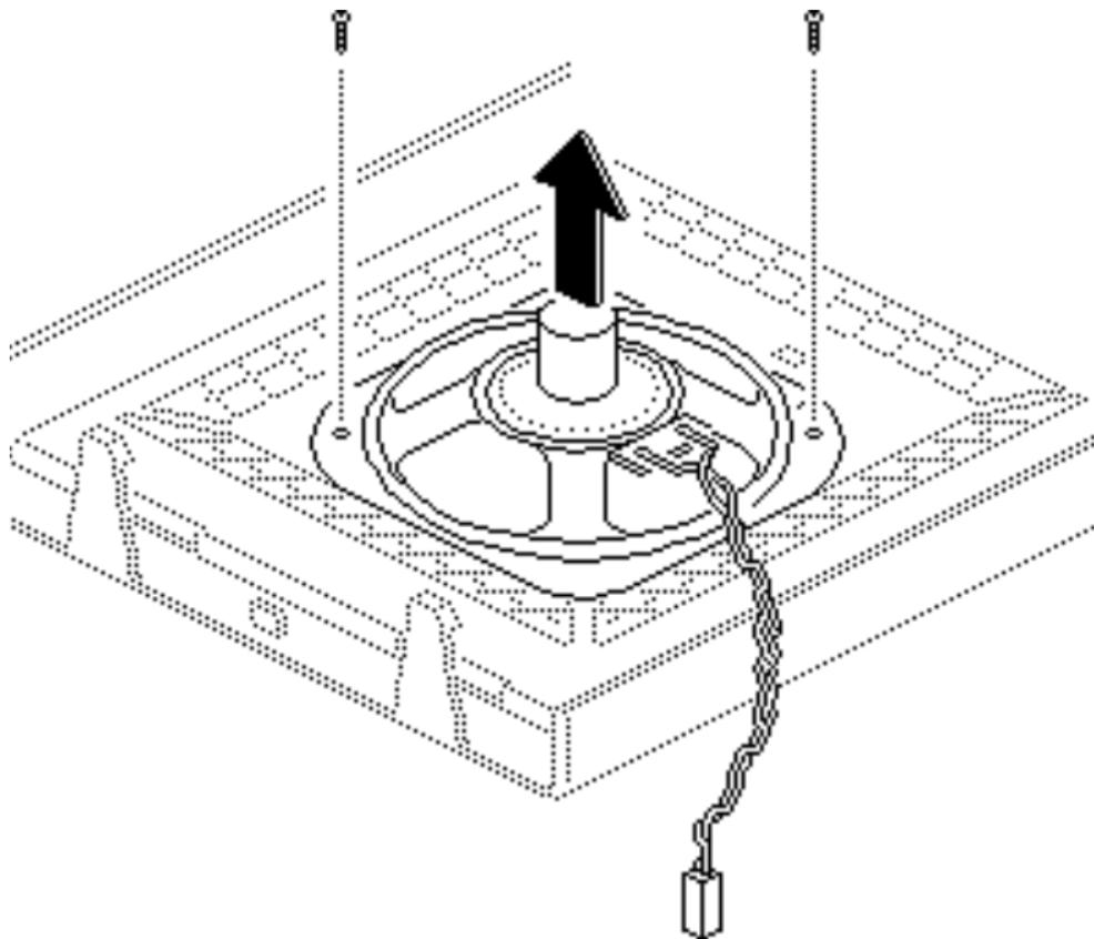
Remove the two screws and lift the speaker off the front panel.
