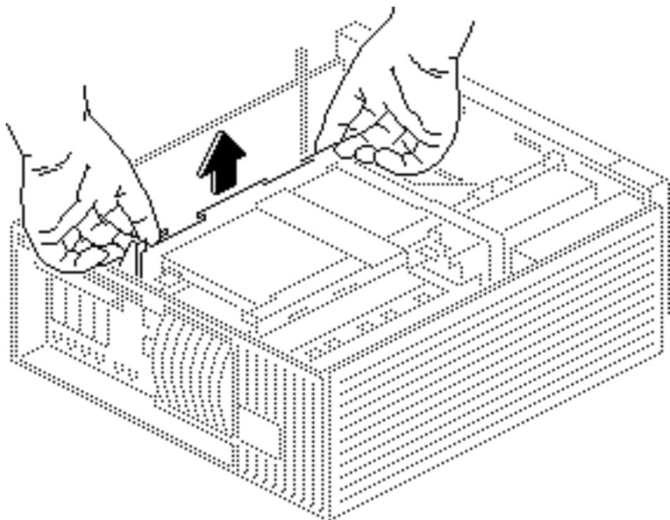
**Caution:** In the next step, pull up evenly on both sides of the card to avoid bending the connector pins.
