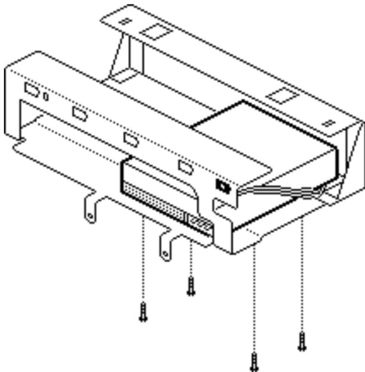
**Note:** Remove the terminating resistors from the drives before installation.
