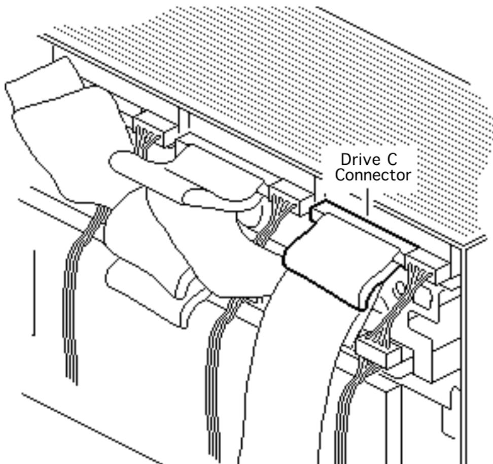
25 Fold over the cable and attach the drive C connector to the drive in slot C.
