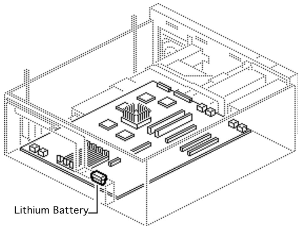
**⚠ Warning:** If handled or discarded improperly, the lithium battery in the computer could explode. Review battery handling and disposal instructions in Bulletins/Safety.
