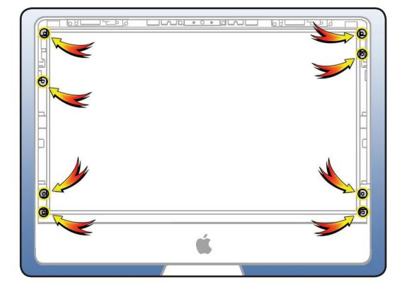
**2** With computer standing up and facing you, pull the LCD forward slightly from the top edge.
