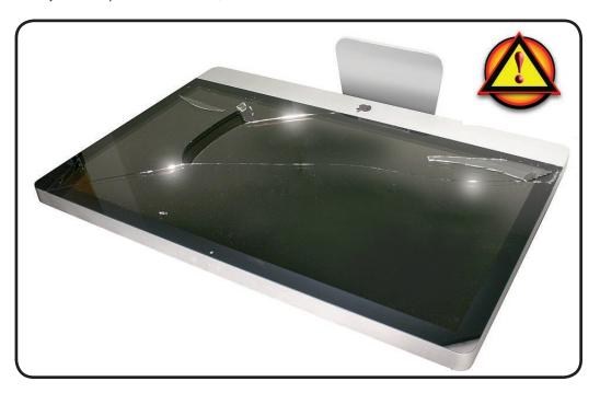
3. Peel protective covering off the front of the glass. Remove and discard any large pieces of broken glass.
