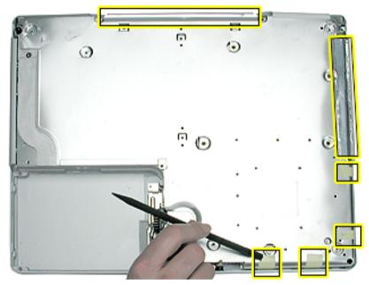
3. Carefully peel up the foil tape at the computer latch. Use the tape when reassembling the computer.
