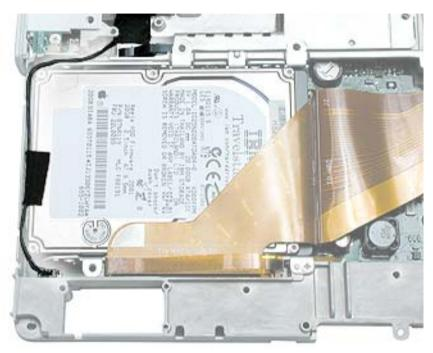
2. Pull up the flexible tab to disconnect the LVDS (low voltage data signal) cable from the logic board.
