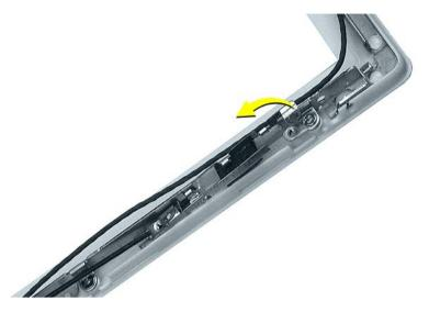
9. On the left side of the bezel, remove the two 3-mm long Phillips screws at the antenna receptor.
