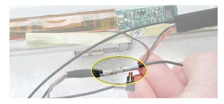
11. Unwrap the tape that secures the AirPort Card antenna to the cable bundle.
