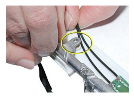
6. With the antenna board loosened, note the cable routing on each side of the bezel. On the right, the antenna receptor cable is routed underneath the microphone cable through two channels before terminating at the receptor bracket.
