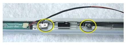
10. Tilt up the antenna receptor to remove it from the left side of the bezel assembly.
