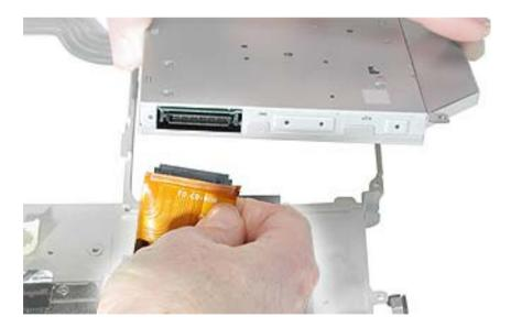
13. Remove the two screws that hold the mounting bracket to the optical drive.
