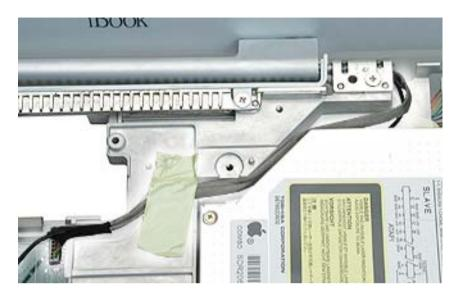
9. Warning: Handle the optical drive at the sides only. Do not touch or press anywhere else on the drive.
