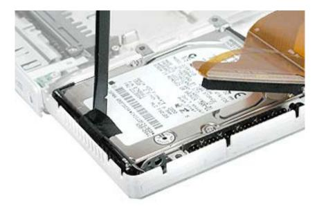
5. From the corner bracket, tilt up the hard drive, and slide it out from under the microphone cable.
