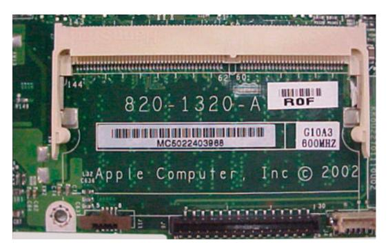
2. If the EEE code begins with the letter "R," replace the board with the matching board shown in the following table:
