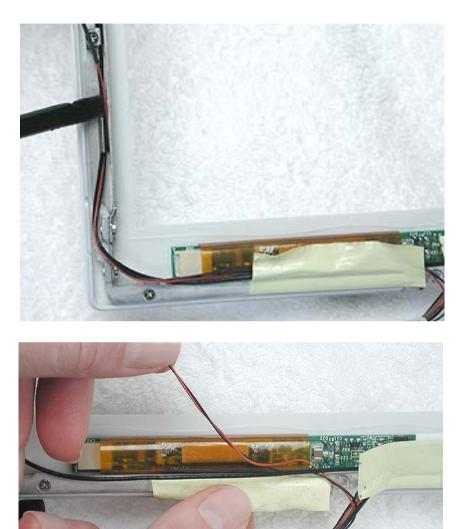
4. Warning: When removing the tape that bundles the reed switch cable assembly to the AirPort Card antenna cable, be careful not to strain or pinch the cables.
