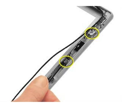
8. Tilt up the antenna receptor to remove it from the bezel assembly.
