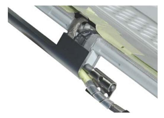
Make sure the clutch cap on each side of the clutch cover is firmly seated before installing the two screws.
