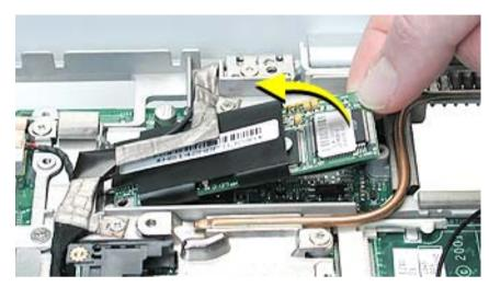
4. Tilt up the end of the modem board to disconnect it from the logic board.
