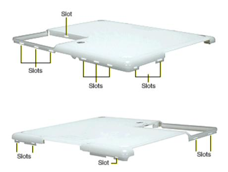
8. In the battery compartment, lift up the corner of the bottom case, and use a black stick or jeweler's flat-blade screwdriver to gently pry up the slot from the inner tabs on the frame.
