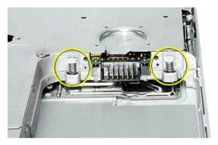
7. Install the replacement bottom shield, and reassemble and test the computer.
