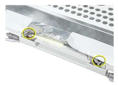
10. Loosen the remaining tape that secures the shield to the assembly. Remove the shield.
