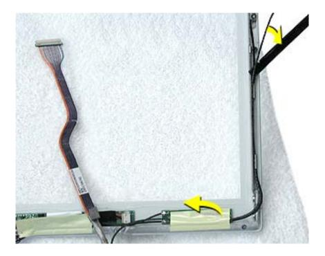
5. Warning: When removing the tape and spiral tube that bundles the microphone cable to the LCD cable, be careful not to strain or pinch the cables.
