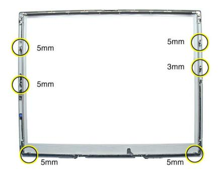
5. Lift the 3-sided bezel brace with clutch assembly off of the bezel.
