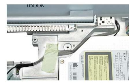
7. Route the cables up through the channel past the optical drive.
