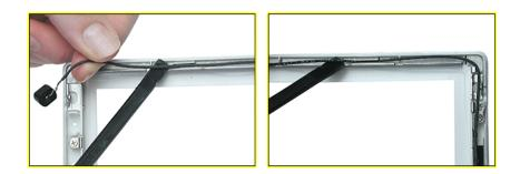
4. Free the microphone cable from the right corner of the bezel and from underneath the tape at the antenna board.
