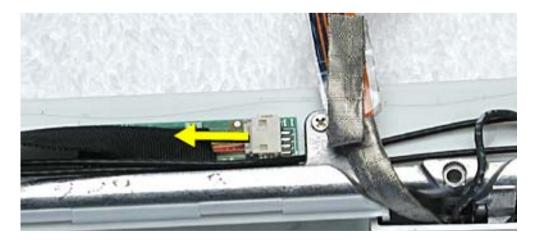
6. Remove the reed switch cable assembly.
