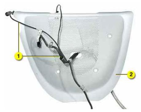
**Note:** Remove five clips from the video cables before returning a faulty cable to Apple. Note the position of the clips in the photo below.
