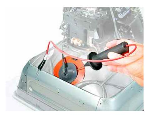
3. Fold up the anode cap, then squeeze together the metal clip to remove it from the internal edge of the anode aperture.
