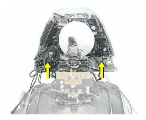
**Replacement Note:** When replacing the deflection board and mount assembly on the CRT, place the edge of the stand tilt base in the bezel channel as shown below.
