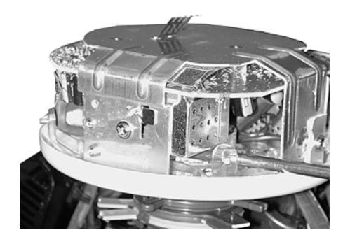
3. Pull the video assembly straight up and off the neck of the CRT.
