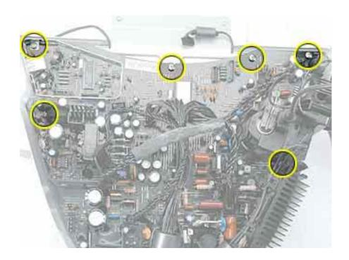
5. Remove the analog board from the PCB mount and place it nearby on the workbench. **Caution:** Note that video cables still connect the anode board and PCB mount.
