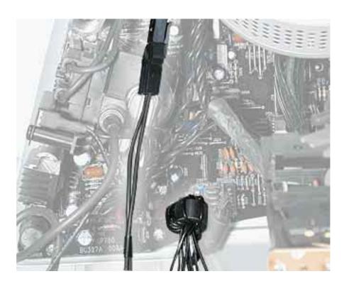
11. Remove the deflection board and mount assembly from the CRT and place it on the workbench.
