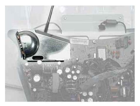
4. Remove the six remaining screws from the analog board and PCB mount.
