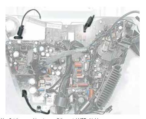
3. Use flat-tip screwdriver to pry off the metal USB shield.
