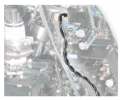
7. Disconnect two anode cables from connectors at the rear of the CRT/yoke board.
