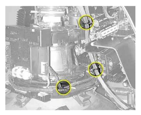
6. Disconnect the degauss cable from deflection board connector B981.
