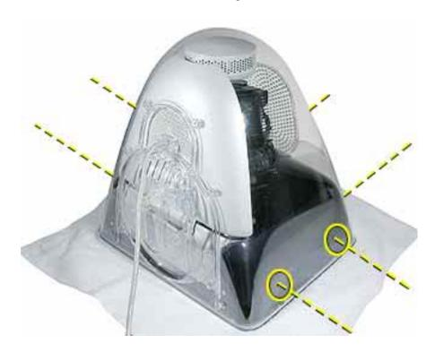
2. Remove four short hex screws (1) and two longer hex screws (2) from the rear of the housing and the stand tilt base.
