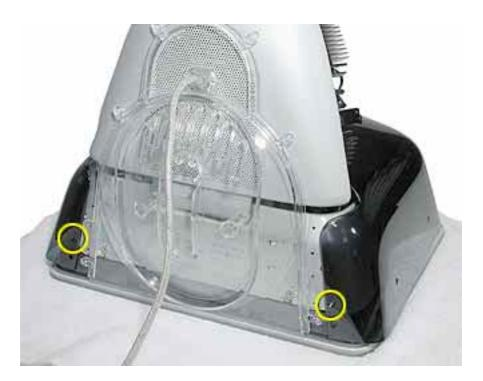
2. Bow out slightly the bottom of the shroud and remove it from the CRT as shown.
