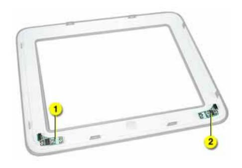
3. Remove two screws and the launch button board (2) from the bezel.
