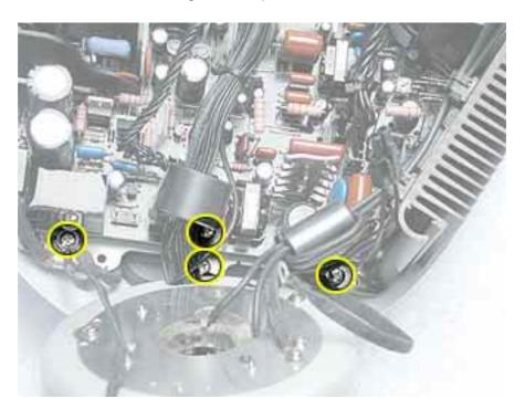
**Replacement Note:** Attach ground straps to the outside mounting screws, and attach a ground strap and clip to the lower, center mounting screw.
