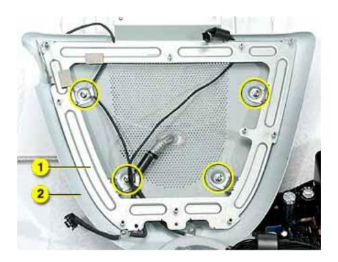
2. Turn over the bottom pan, and separate the stand tilt base (1) from the bottom pan.
