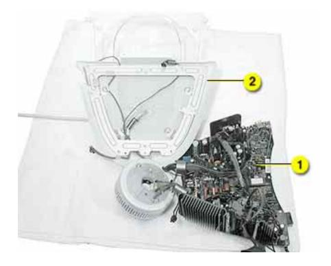
6. Remove the screw and ground cable from the bottom of the video shield. Remove two of the remaining three screws as shown. **Note:** Do NOT remove the last screw, shown in red below.
