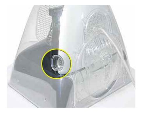
**Replacement Note:** Replace the USB label. The USB label should not be re-used because the adhesive may not hold the label properly.
