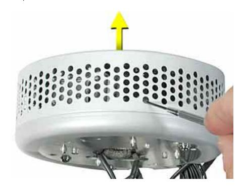
2. Use #2 Phillips screwdriver to loosen the neck clamp as shown below.
