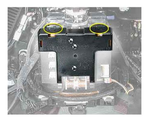
9. Remove two screws and four ground cables from the the video shield.
