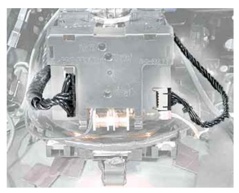
8. Using a small, plastic flat-blade screwdriver, release two tabs at the top of the CRT/ yoke board cover and separate the cover from the CRT/yoke board.
