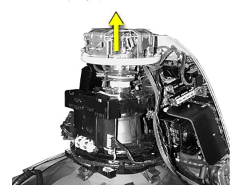
**Replacement Note:** Visually inspect the pins on the CRT and straighten any that are bent. Carefully align and position the video assembly connector on the neck of the CRT before pressing it down firmly.
