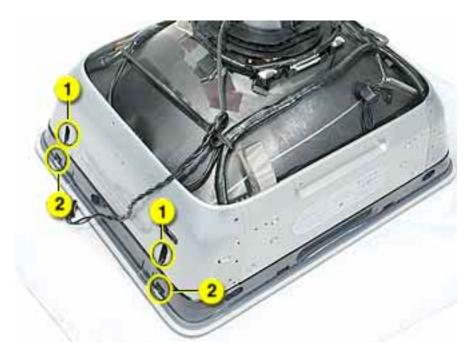
2. Lift slightly the bottom side of the degauss frame and disconnect the power button cable and the launch button cable. Remove the CRT from the front bezel assembly.
