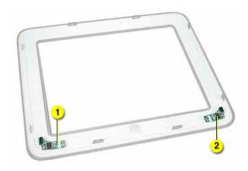
4. Remove the power button (1) and the launch button (2) from the front bezel.
