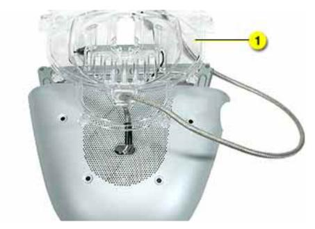
3. Pull the video cable off the bottom pan and pop open the plastic strain reliefs.
