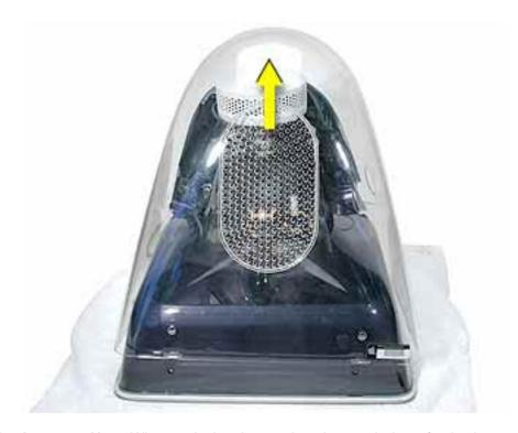
**Replacement Note:** When replacing the rear housing, push down firmly along each side of the housing until you hear it snap securely onto the bezel.
