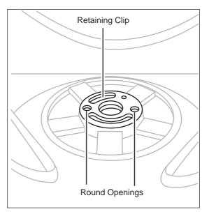
5. Using two jeweler's flat-blade screwdrivers, place one in each of the round openings and gently pry up the retaining clip until it is out of the monitor stand.
