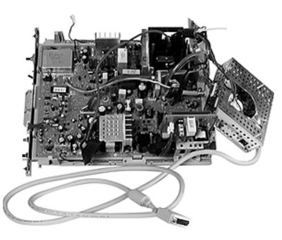
**Replacement Note:** Avoid pinching or straining cables when replacing the main deflection board and CRT/ video board module.
