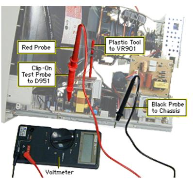
10 Turn on the voltmeter and use the plastic tool (nonconductive screwdriver) to adjust VR901 so that the voltmeter reads a voltage of 175 VDC  $\pm$  0.5 V.
