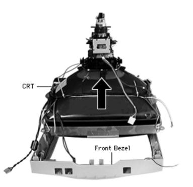
3 With both hands, grasp the CRT by its edges and lift it off of the front bezel.
