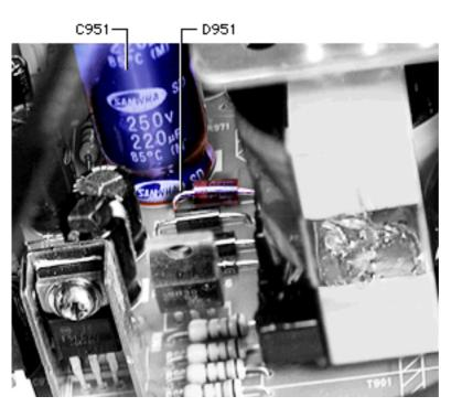
2 Locate diode D951 on the main deflection board (near capacitor C951.)
