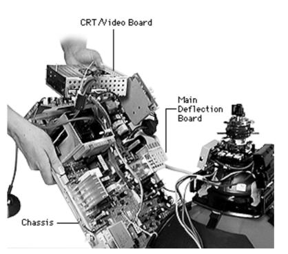
11 Lift the main deflection and CRT/video board module away from the CRT.
