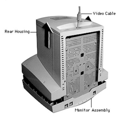
2 Lift the rear housing straight up from the monitor assembly. Feed the video cable through the opening in the rear housing.
