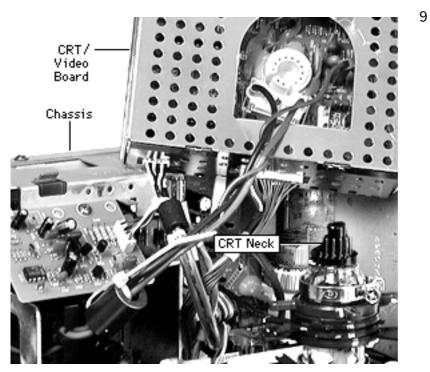
With the CRT/video board wires still attached, remove the CRT/video board from the CRT neck, and rest it on the main deflection board chassis.
