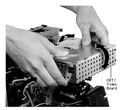
8 **Caution:** CRT pins are easily damaged. Gently rock the CRT/video board back and forth while pulling it away from the CRT.
