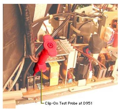
3 Attach a clip-on test probe to the cathode (striped end) of diode D951.
