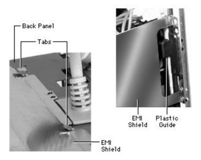
**Replacement Note:** Before replacing the EMI shield screws, ensure the shield is fitted between the two tabs on the back panel and the plastic guides on the chassis sides.
