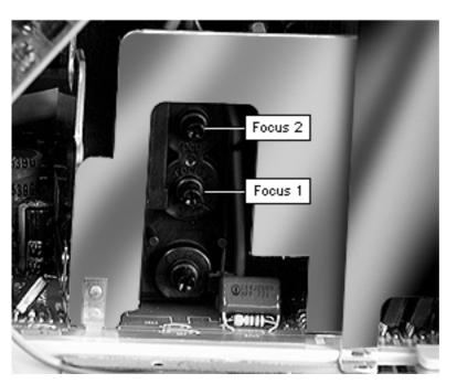
5 Use a plastic screwdriver to adjust the two Focus controls on the flyback transformer for best center screen focus.
