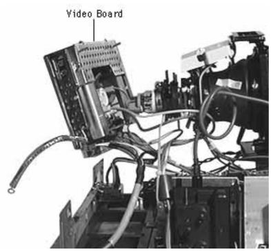
**Caution:** CRT pins are easily damaged. Gently rock the video board back and forth while pulling it away from the CRT.
