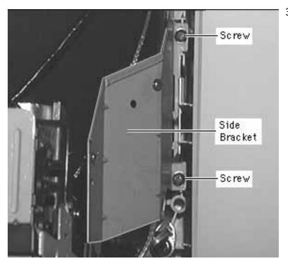
3 Remove four screws (two each bracket) securing the left and right side brackets to the bezel.
