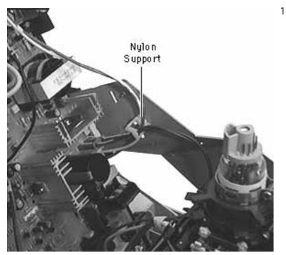
Remove all wires from the nylon support on the right side bracket.
