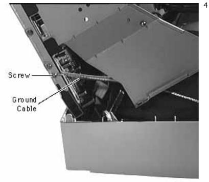
4 Remove two screws securing the ground straps to the bottom bracket.
