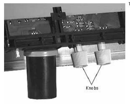
17 Remove the user brightness and contrast knobs from the controls on the main deflection board.
