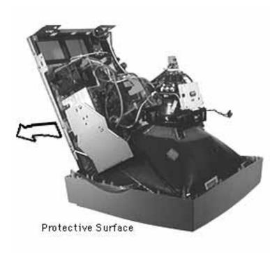
12 Lift and tilt the video and main deflection board assembly away from the CRT.
