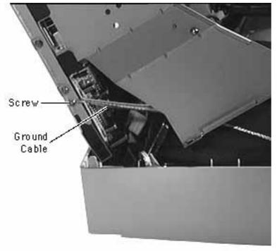
**Caution:** Ground cables are supporting the weight of the video and main deflection board assembly. Support this assembly with your hand when removing the ground cables.
