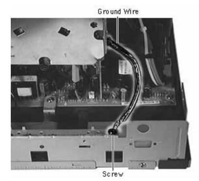
10 Remove the screw securing the video board ground wire to the fence
