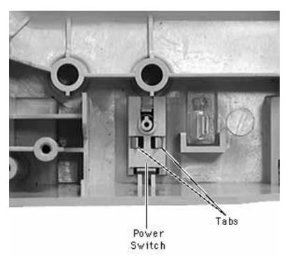
**Note:** The switch is spring loaded and will fly when pushed from the bezel.
