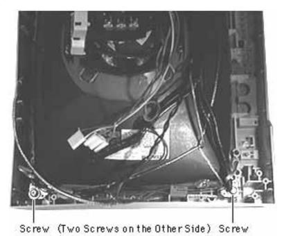
7 Remove the four screws securing the D-coil holders and CRT to the bezel.
