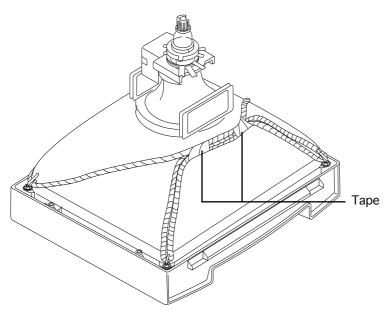
3 **Note:** Do not remove the board assemblies. The illustration at left shows the boards removed for clarification only.
