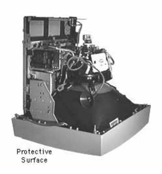
**Caution:** When the monitor is face down, it is resting on the CRT screen. The CRT must rest on a protective, nonabrasive surface or the screen will become damaged.
