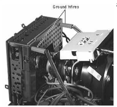
2 Disconnect two ground wires from the video board.
