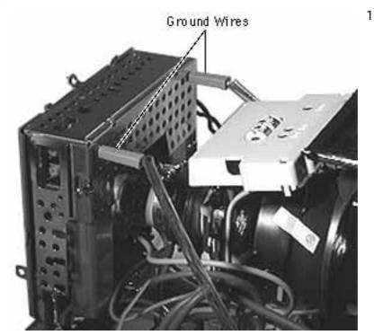
Remove two ground wires from the top of the video board.
