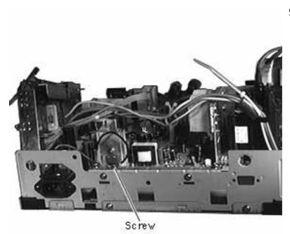
9 Remove the screw securing P704 cable to the rear fence.
