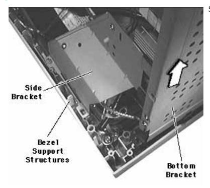
5 Gently lift the right side of the bottom bracket so the side bracket just clears the bezel support structures.
