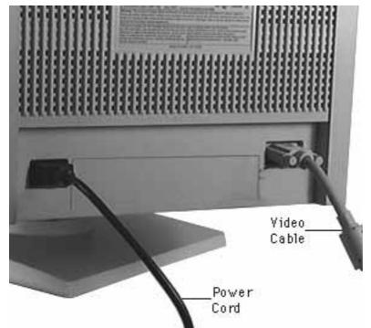
1 Remove the power and video cables from the monitor.
