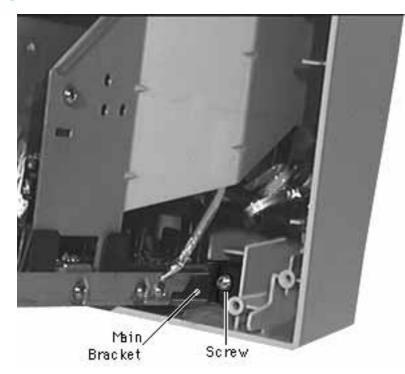
4 Remove two screws securing the main bracket to the bezel.
