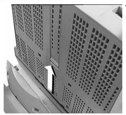
4 Slide the monitor stand toward the back of the monitor and remove.
