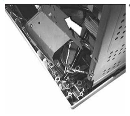
6 Slide the side bracket from the main bracket support and remove.
