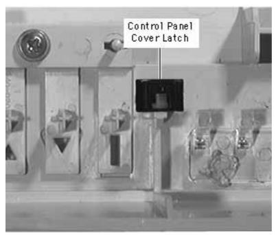
3 With an object about one-half inch in diameter and three inches long, drive the latch from the inside of the bezel.
