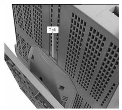
3 Depress the tab on the rear of the housing, just behind the monitor stand.
