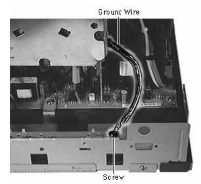
5 Remove one screw securing the ground wire to the rear fence.
