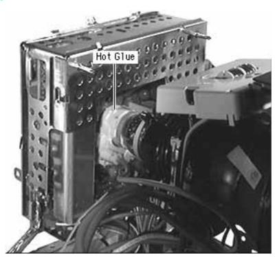
**Caution:** Damage will occur if the CRT is marred with pliers when removing the hot glue.
