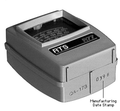
readings, verify the readings with a known-good light meter or photometer. Also check the age of the R77 light meter by its four-digit manufacturing date stamp (such as 0398 for March 1998).
