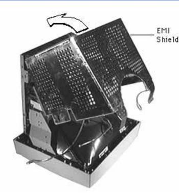
6 Tilt the EMI shield so the shield tabs clear the slots in the rear fence and lift off.
