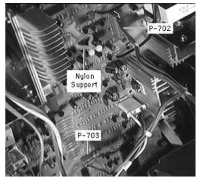
6 Remove the cable from the nylon support.
