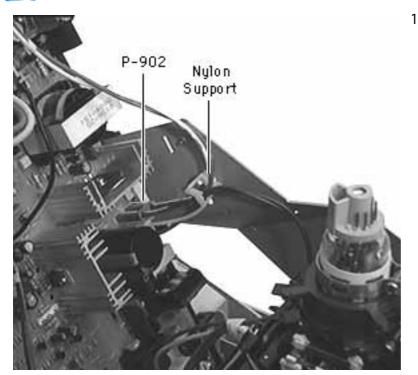
15 Disconnect the twowire cable from P902 on the main deflection board and remove both cables from the nylon support.
