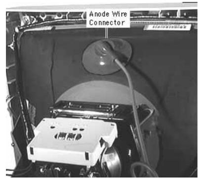
**Warning:** Be sure the monitor has no power and the CRT has been properly discharged. Serious injury could occur if the anode wire is removed while the CRT is charged.
