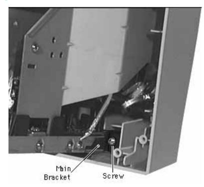
11 Remove two screws securing the main bracket to the bezel.
