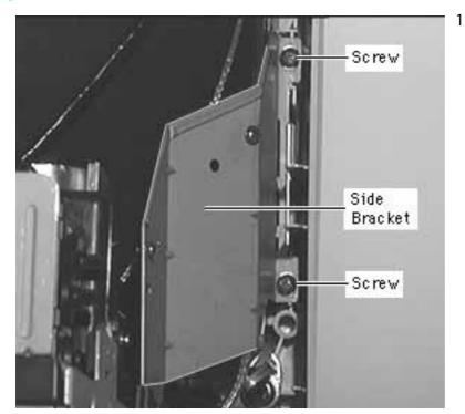
10 Remove four screws (two each bracket) securing the left and right side brackets to the bezel.
