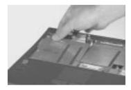
3. Use this special tool placing it under the CPU board and aligning it with the white line, then lift up the CPU board to bring it out from the system board.
