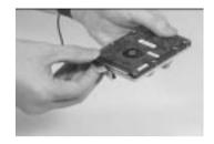
5. To reconnect the hard disk cable, be sure that the 1st pin is aligned up as indicated.
