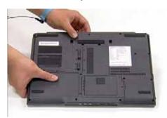
3. Engage the battery lock as shown.
