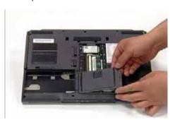
2. Replace the two screws to secure the cover in place.
