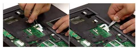
**2.** Disconnect the second cable by releasing the locking latch and removing the cable as shown. **NOTE:** Move the cable away from the work area to allow access to the third cable.
