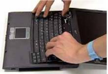
**4.** Push the Keyboard into place toward the TouchPad and secure using the two screws provided.
