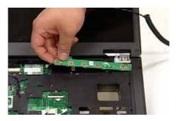
2. Secure the Switch Board in place using the screw provided.
