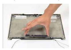
**6.** Grip the WebCam Module and lift upward to remove.
