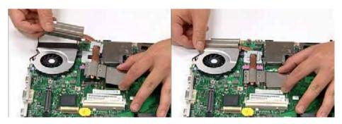
3. Align the Heatsink Securing Bracket as shown.
