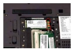
3. Reconnect the three Antenna Cables as shown, pushing down firmly to connect the cables.
