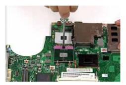
2. Remove the CPU from the bracket as shown.
