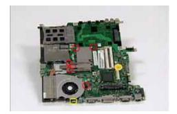
2. Remove the Heatsink securing bracket as shown.
