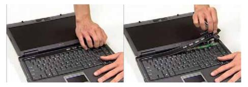
**4.** Using two hands, remove the Switch Cover from the chassis.
