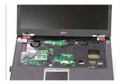
3. Lift the LCM Module upward to remove from the chassis.
