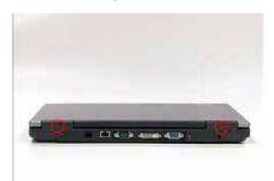
2. Open the LCM module fully to expose the Switch Cover.
