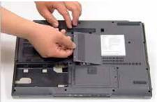
4. Remove the HDD cover as shown.
