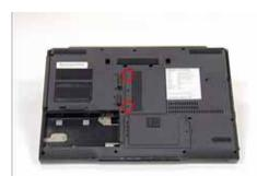
5. Replace the seventeen (17) screws to secure the cover in place.
