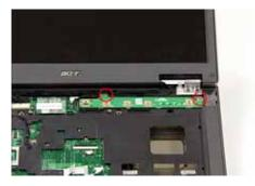
2. Remove the Switch Board from the chassis.
