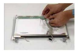
9. Locate and remove the four screws (two on each side) securing the LCD brackets to the LCD panel.
