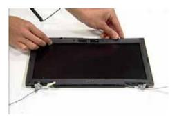
**5.** Remove the bezel from the LCM Module.
