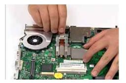
**4.** Secure the five screws and fan connector as shown.
