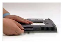
3. Locate Dummy Tray 2 and press the release button as shown.
