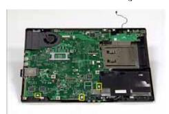
2. Disconnect the connectors using tweezers as shown.
