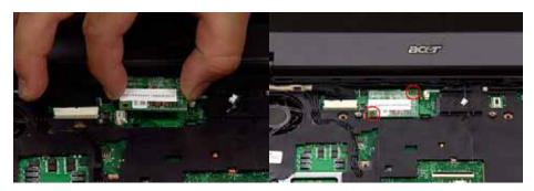
2. Reconnect the Modem cables as shown.
