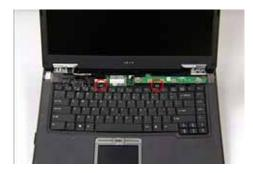
5. Turn the Computer over and insert the screw as shown.
