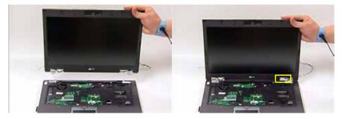
2. Secure the four screws to hold the LCM in place on the chassis.
