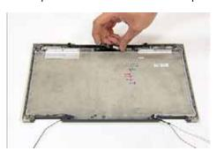
7. Turn the LCD panel over to expose the rear. Grip the LCM cable and lift upward to detach the adhesive pads.
