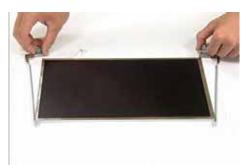
2. Secure the LCD brackets to the LCD panel.
