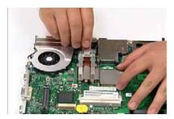
3. Remove the Heatsink as shown.
