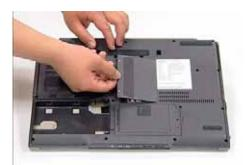
**4.** Replace the two screws to secure the cover in place.
