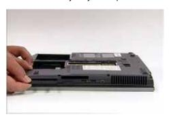
2. Insert Dummy Tray 1 and push into the slot until flush with the chassis cover.
