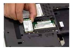
2. Secure the card in position using the two screws provided.
