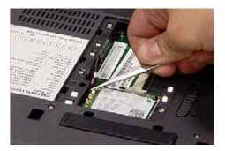
2. Using fine tweezers, grip the white taped wire and pull upward until it is released from the board.
