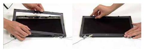
2. Secure the six screws provided and replace the mylar (small red markers) and rubber screw caps (large red markers).
