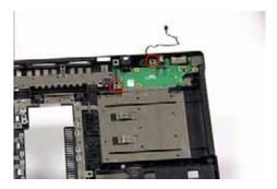
2. Lift the board toward the front of the computer to clear the port and remove from the chassis.
