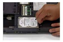
3. Pull away from the connector and upward as shown to remove the HDD from the chassis.
