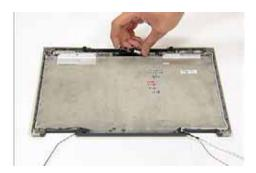
**6.** Place the Inverter Board in the mounting and secure with the screw provided.
