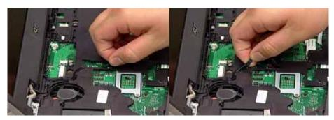
2. Pull the three Antenna Cables from the underside of the computer through the mainboard as shown.
