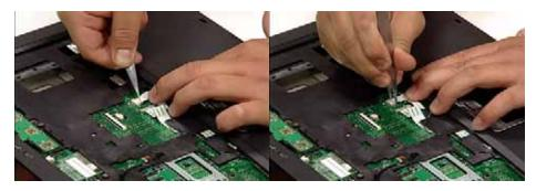
3. Insert the second cable as shown and lock the latch to secure the cable in place.
