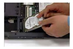
2. Push firmly toward the connector to secure the HDD.
