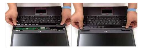
2. Close the LCM Module. Locate and replace the two screws as shown.
