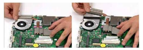
4. Steady the Mainboard with one hand and remove the Fan Module by lifting straight up.
