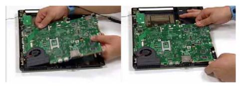
2. Replace the three connectors in the Mainboard sockets as shown.
