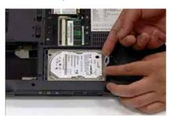
2. Place one hand on the computer for stability and grasp the HDD removal tag.
