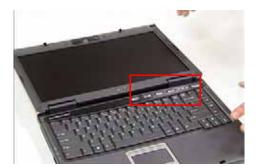
3. Grip the Switch Cover as shown and pull upward to remove.
