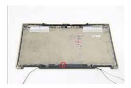
5. Grip the Inverter Board and lift upward to remove.
