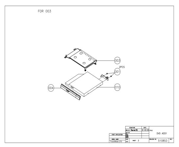
**NOTE:** The exploded diagrams for CD-ROM, DVD-ROM and DVD-RW combo module are very similar. Therefor, we put only DVD ASSY exploded diagram for your reference. Please also refer to the FRU list below for more information on different models and part numbers. This diagram only explains the relevant location of each part. The parts on the exploded diagrams may be a slightly different from its actual looks.
