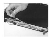
5. Disconnect the LED cable from the LED board.
