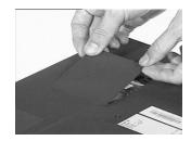
2. Use two flat-bladed screwdriver to push the latches outward on both sides of the DIMM socket to remove the DIMM module from the DIMM socket
