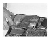
2. Disconnect the CD-ROM cable at CN18 and diskette drive cable at CN17 from the system board.
