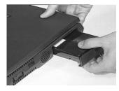
2. To remove the battery cover, gently bend the battery cover a little bit outward, then slide the battery cover downward to remove it.
