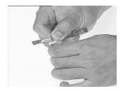
6. Carefully remove the internal microphone cable from the LCD panel.
