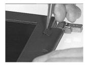
2. Remove the five screws from the LCD bezel as shown below.
