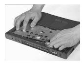
3. Remove the CPU EMI Shield from the system board.
