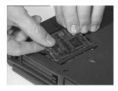
3. Disconnect the modem power cable from the modem board.
