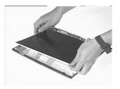
8. To remove the LCD inverter board, disconnect the LCD power cable and LCD FPC cable from the inverter board.
