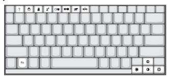
The computer employs hot keys or key combinations to access most of the computer's controls like screen contrast and brightness, volume output and the BIOS setup utility.
