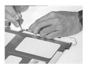
9. Carefully tear off the adhesive tape and remove the LCD FPC cable from the LCD.
