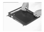
4. Remove the two screws of the LED board, then lift the LED board away from the LCD panel..
