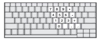
The embedded numeric keypad functions like a desktop numeric keypad. It is indicated by small characters located on the upper right corner of the keycaps. To simplify the keyboard legend, cursor-control key symbols are not printed on the keys.
