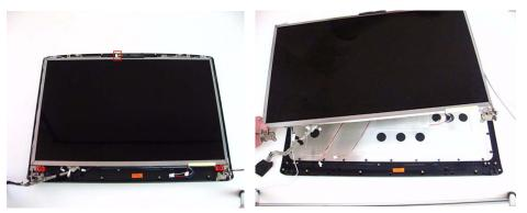
9. Loose four LCD hinge screws, then remove two hinges from LCD panel.
