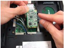
8. Remove HDD module as shown.
