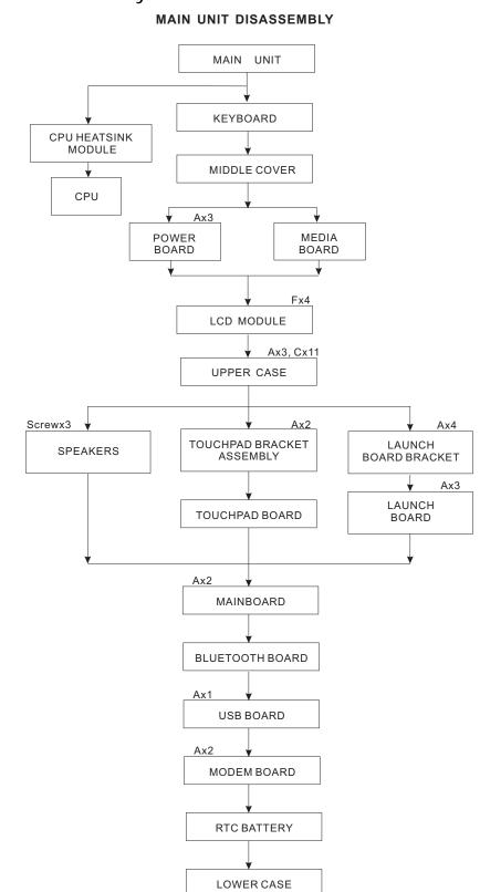
Main Unit Disassembly Flowchart
