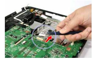
16. Pull out the AC input cable and move away from the USB board.
