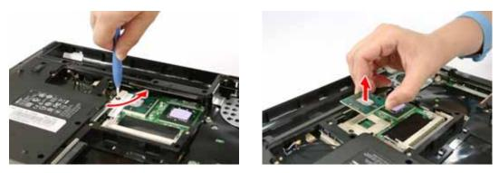
NOTE: When installing the CPU, make sure to install the CPU with PIN 1 at the corner as shown.
