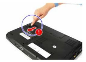
3. Slide and hold the battery release latch to the release position (2).
