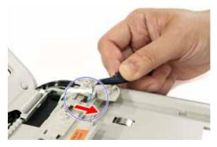
7. Detach the power board cable from the power board, then remove the middle cover.
