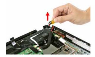
17. Remove the screw (A) on the USB board.
