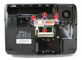
5. Remove the heatsink module.
