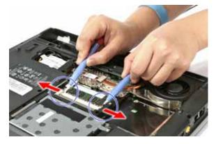
4. Remove the DIMM module.
