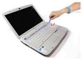
3. Carefully pry up and out the keyboard and turn it over.
