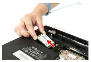
NOTE: When attaching the antennas back to the WLAN board, make sure the cable are routed properly.
