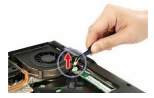
4. Loosen the four spring-loaded screws on the heatsink in the order shown.
