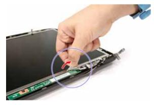
14. Remove the screw (G) that holds the board to the panel.
