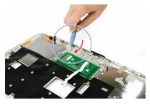
18. Continue prying the board until it releases from the upper case, then remove the board.
