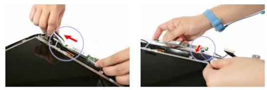
**17.** Remove the inverter board.
