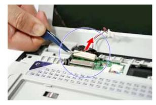
7. Pull out the antenna cables as shown.
