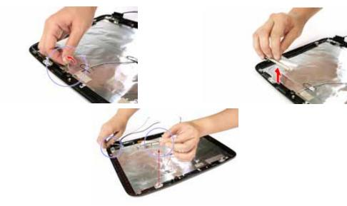
**16.** Detach the gasket tape holding the left antenna in place, remove the antenna bracket, then carefully remove the antenna.
