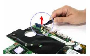
**19.** Detach the masking tape from the mainboard.
