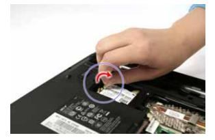
4. Disconnect the two antenna cables from the WLAN board, then move the antennas away from the board.
