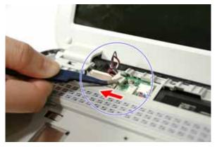
6. Disconnect the LCD coaxial cable from the mainboard.
