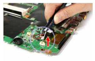
**19.** Carefully detach the RTC battery from the SD card slot.
