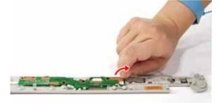
5. Remove the three screws (A) from the power board.
