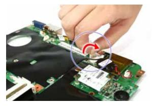
**20.** Remove the two screws (A) on the modem board.
