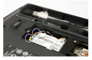
5. Remove the two screws (A) on the WLAN board to release the WLAN board.
