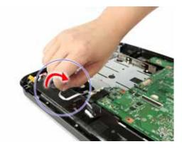
**18.** Detach the power board cable from the lower case.
