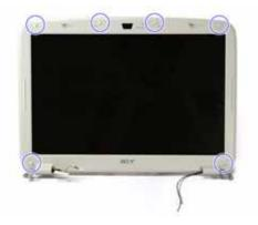
**13.** Remove the six screws (G) on the LCD module.
