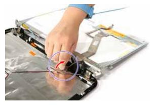
17. Detach the acetic tapes holding the FPC cable to the edge of the LCD panel.
