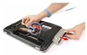
5. Remove the two screws (D) securing the optical bracket and remove the locker bracket from the optical disk drive module.
