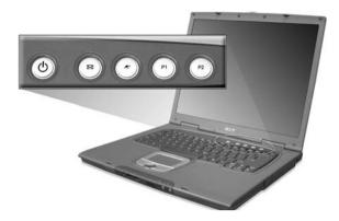
**NOTE:** To the left of these five launch keys is the wireless communication button. This wireless communication button works for model with 802.11b wireless LAN only.
